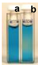
Figure I.3 – Gelatine indigo carmine gel before a) and after b) 335nm irradiation.
