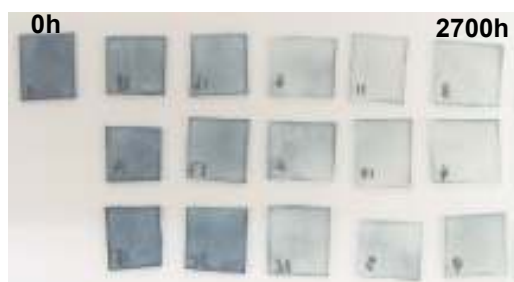
Figure I.4 – Indigo cells irradiated in the solar box.
