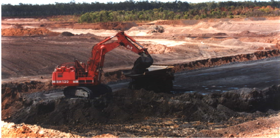
Figure 2-7 Mine pit with the O&K excavator loading manganese ore into a Komatsu 785 haul truck
