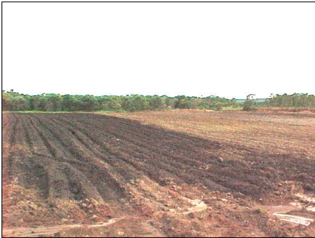
Figure 5-3 Substrate trial after ripping, viewed from the south east, with the direct-return topsoil treatment in the foreground
