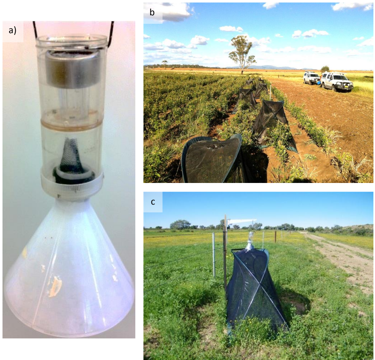
Fig. 11. First iteration of field emergence cages used in the Namoi Valley and inland Queensland. Fig. a) shows the detail on the capture mechanism, two plastic culture tubes glued together, with an ultraviolet LED wired into a solar-array that activated after dark. A 45mm powder funnel was attached to the bottom culture tube via the lid of the culture tube and a rubber washer. One-way glass fibre mesh prevented moths from escaping the culture tube. Fig. b) shows the offset cages that the capture mechanism was used in, at Boggabri NSW. Fig. c) shows how the capture mechanism was attached to the cages, via an iron post, tensile cord and metal bracket.
