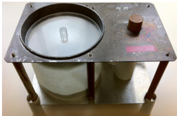
Fig. 3. A mating cage used to obtain H. punctigera eggs by placing adult moths inside the chamber for a 3-5 day period. The paper sides of the cage were scrolled to obtain eggs while keeping the adults in the cage.
