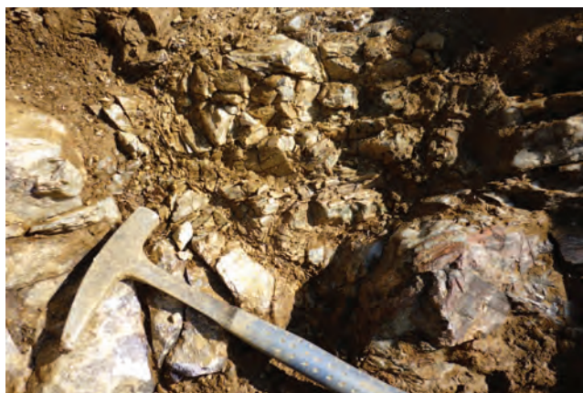
Figure 4. Lens of fractured and altered, white to pink spodumene in situ , in the trench after washing and scrubbing to remove mud, clay, etc. The hammer head is 15 cm in length.
