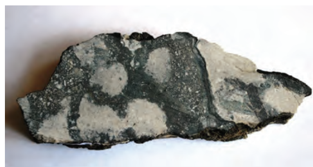
Figure 5. Cut surface of magnetite concentrations surrounding marble cores in altered pseudobreccia. Note the abundant white crinoid ossicles contrasting with the surrounding dark grey magnetite. Dump from White Force Level – Location 4. Specimen is 14 cm across. B. Young Specimen No. BY8485/B; Jane Young photograph.
