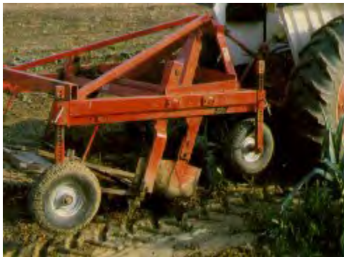
Figure 3. A vibrating lifter loosens plants and removes a large part of the soil from the roots.
