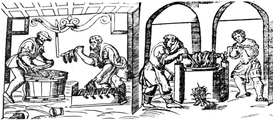
Dyeing skeins (left) and fabrics in heated dye bath(right) from 『 Plichto 』, Venice, 1540 (Edelstein, 1955).
