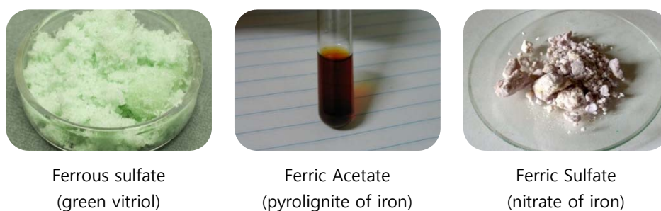
Figure 11. The most common types of iron mordant used in 18-19 th C. (Library; Wikipedia; Wikipedia)
