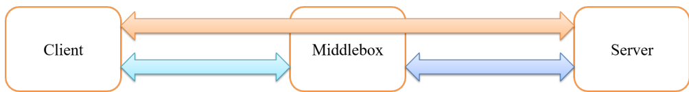
Figure 2.3: In-band Channel Approaches Middleboxes intervene in the session by actively participating in the negotiation with endpoints and other middleboxes.
