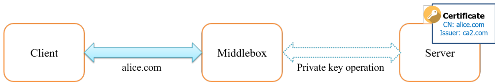
Figure 2.6: Key Server-based Approaches A server performs a private key operation on request from a middlebox; thus, a server does not need to delegate a private key to a middlebox.
