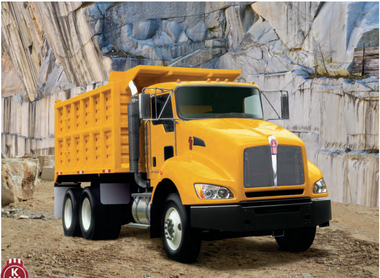
The robust Kenworth T460, featuring a set-back front axle, a tight turning radius and an optional automatic transmission, is agile, comfortable and easy to operate – perfect for Mexico’s vocational applications.
