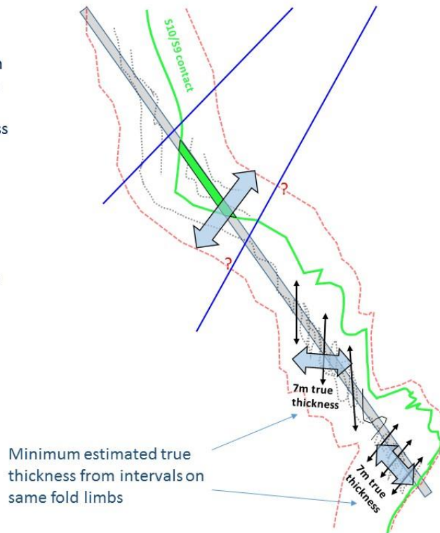
Figure 10.6 - Example of true thickness estimation methodology for Amaruq
