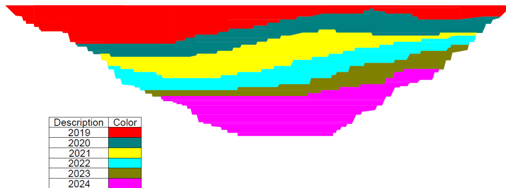
Figure 16.9 - Schematic mining for Whale Tail pit
