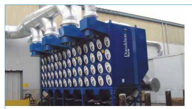
Our Donaldson<sup>®</sup> Torit<sup>®</sup> Downflo<sup>®</sup> Oval Dust Collector at a titanium grinding operation
