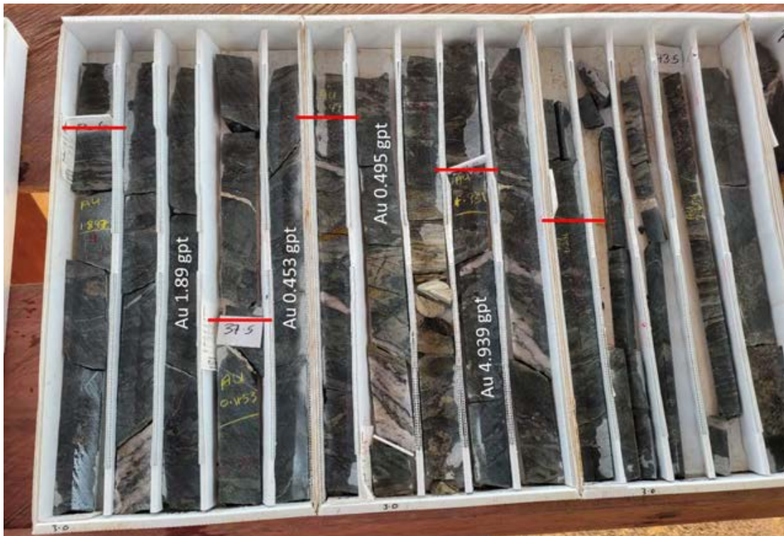
Figure 12-15: DDH TPD325 between 35.5 m and 44.06 m outlining gold grades over an interval of approximately 8.56 m
