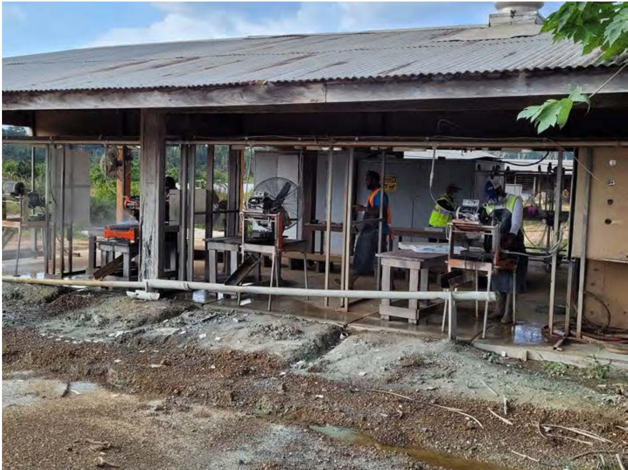
Figure 11-1: Core being halved by diamond saw and sampled with pre-marked sample bags.
