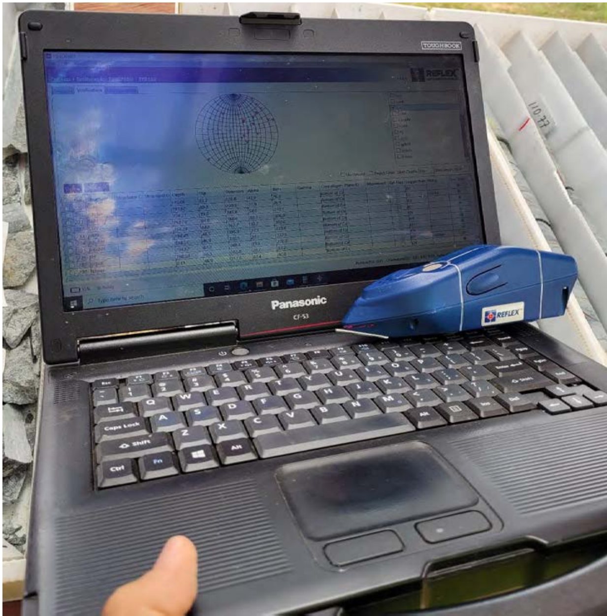
Figure 12-2: Reflex IQ Logger, collection of structural measurements
