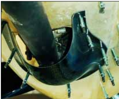
A scratch-built carbon-fiber exhaust cover hides the elbow of the Sky Raider's Rotax 503.
