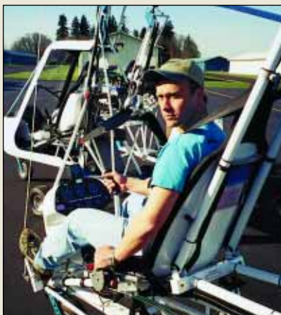
The new two-place tandem is designed so that the front cockpit serves as a "student" seat; Vanek demonstrates.
