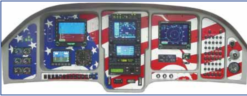
Aerotronics debuted this all-glass Lancair IV-P panel at Sun 'n Fun this year. The main features include the following: (1) Sierra EFIS from Chelton Flight Systems, (2) Dynon D10 EFIS, (3) Sandel electronic HSI, (4) TruTrak DFC-250 or -300 digital autopilot, (5) Garmin 530 and 430 panel-mount GPSs, (6) Garmin GNC 340 audio panel, and (7) Garmin GTX 327 transponder.
