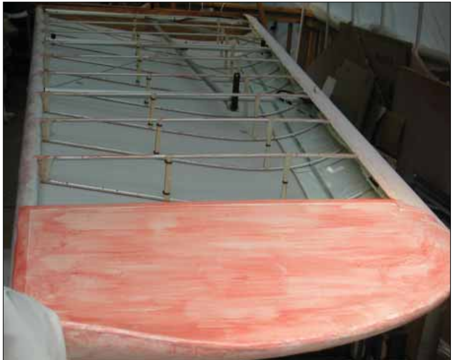
Covering the aircraft according to the Stits Poly-Fiber method proved one of the most enjoyable parts of the project. The first step in the process is to prep the framework with Poly-Brush (the pink stuff).
