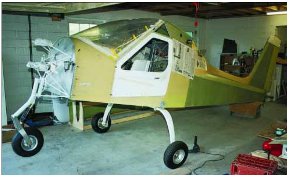
Williams and Franklin called trimming and fitting the Plexiglass windshield the most difficult part of the building process.
