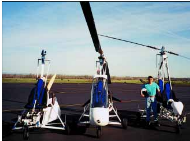
Jim Vanek poses with the company's three current offerings: the two-place Vortex II (right), the single-place Vortex (middle) and the ultralight Lightning.
