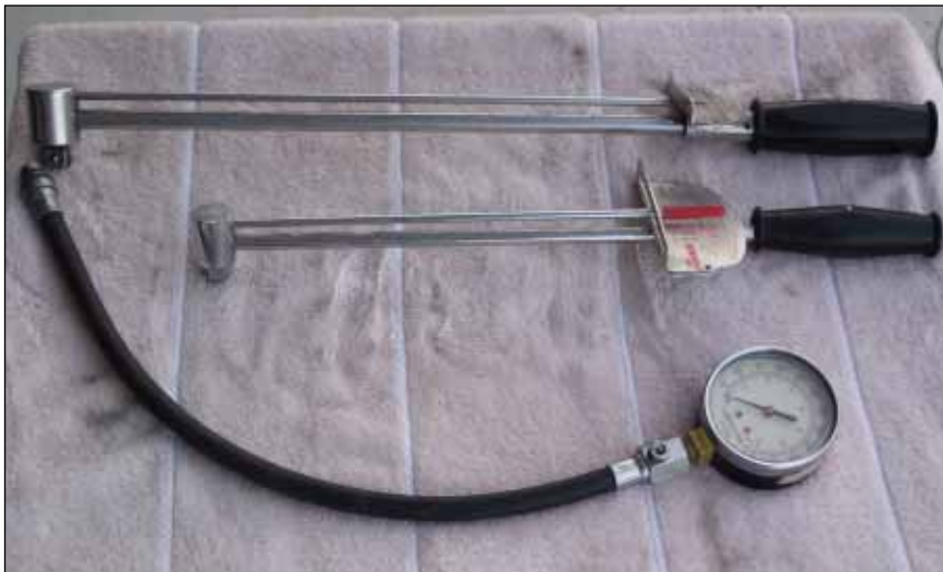
Along with your basic tools, you'll need torque wrenches calibrated in inch-pounds and foot-pounds. A compression tester is mandatory to track the condition of your engine's cylinders.
