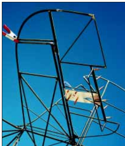
The empennage is of Raeder's own design; he modified the stock design to more closely match that of the Avid Magnum. But for safety, the tail section was welded to the airframe at the Flying K factory.
