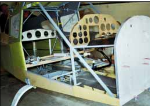
Early in the construction process, the author caught a glimpse of the firewall and partially completed instrument panel and cockpit area.
