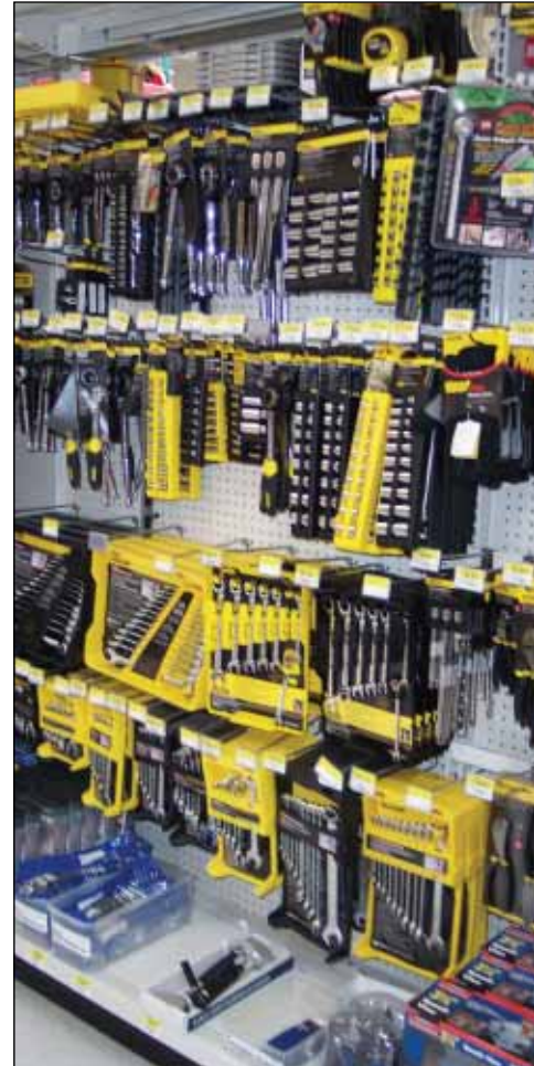
You don't need a store full of tools, but a basic set of wrenches and sockets in both metric and U.S. inch sizes is a must along with good pliers and a screwdriver assortment.
