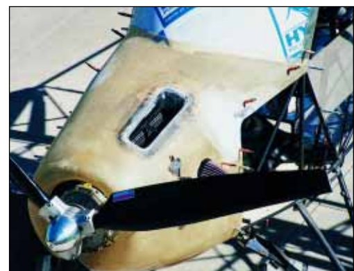
Raeder custom-designed a carbon-fiber cooling-air exhaust port.
