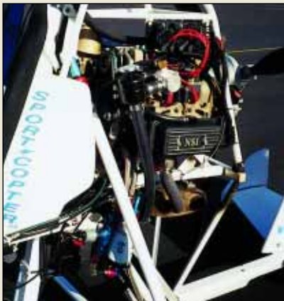
The Vortex II is powered by a 160-hp NSI converted Subaru engine. It allows for a 400- to 500-fpm climb at full power with 430 pounds of useful load.
