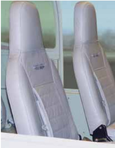
The Oregon Aero High-G Safety Seat is standard equipment for the RV-10's two front seats.
