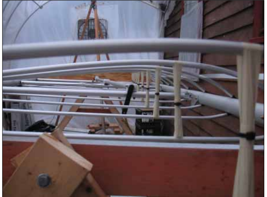
Here's the wing structure—the author riveted the pre-formed aluminum-tube wingribs to the fore and aft wingspars.
