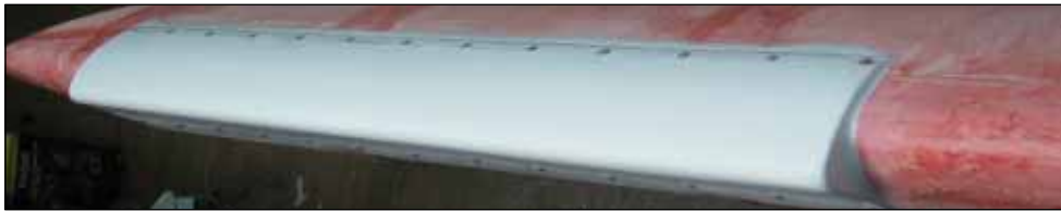
Fiberglass leading-edge extensions attach to each of the SeaRey's wings. These keep the aileron flying until well after the inboard portion of the wing has stalled.
