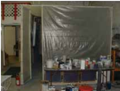
Taking it to the next level—using PVC pipe and plastic sheeting, Gross designed his own homemade spray booth.
