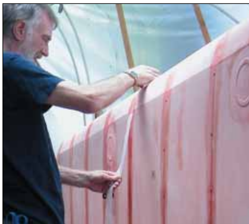
After smoothing out the fabric, the author again went back to ironing, but not before he applied finishing tape over the ribs and seams.
