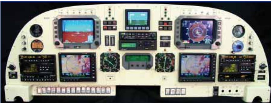
Sterling Ainsworth had Aerotronics create this instrument panel for his IV-P. As you can tell, it would be difficult for a steam-gauge-only pilot to hop in and fly without transition training.
