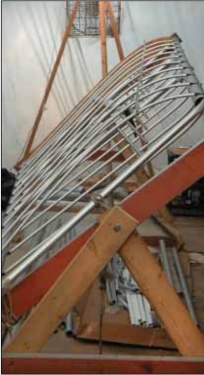
The author built a wing rotator stand of 2x4s to support the root end of the wings.
