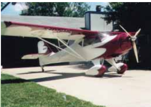
Originally purchasing his Kitfox Speedster as a long-wing model, Bryan Lee Fisher decided to trim down the wing on his plane so he could add more mods to it, such as the Speedster radiator cowl and Speedster wingtips.
