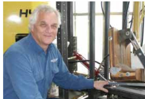
Oregon Aero's high-quality, adjustable test fixture allows checking components (seats and mounting hardware) under high hydraulic load for failure and springiness.
