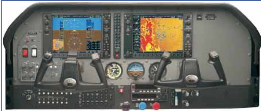
Here's what the G1000-equipped Cessna 182 instrument panel looks like; the screen on the left is the PFD, and to the right is the MFD. Three "steam"-powered instruments remain below the displays for backup.
