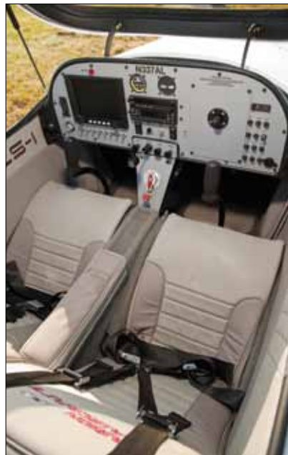
A GRT Avionics EFIS with synthetic vision and an integrated engine monitor anchor the Lightning's panel. Two seats are separated by a thin center console. A clever mixture adjuster (red knob) "fools" the Jabiru's Bing carburetor into reducing fuel flow in cruise.
