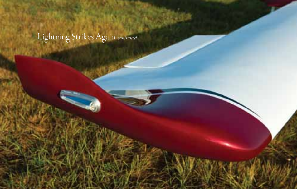
Upswept wingtips help improve aerodynamics and efficiency on the long-wing LSA model.
