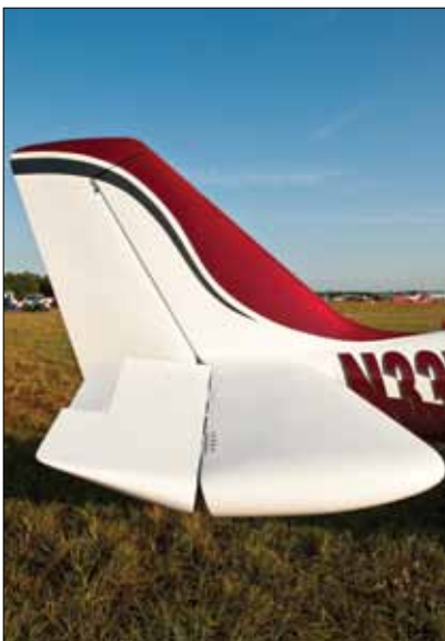
By adding 3 square feet of horizontal stabilizer, Arion's Nick Otterback gave the Lightning substantially improved pitch stability. The maximum throw of the top-hinged elevator was reduced 10° to 15° up. Electric pitch trim remains as a separate tab.
