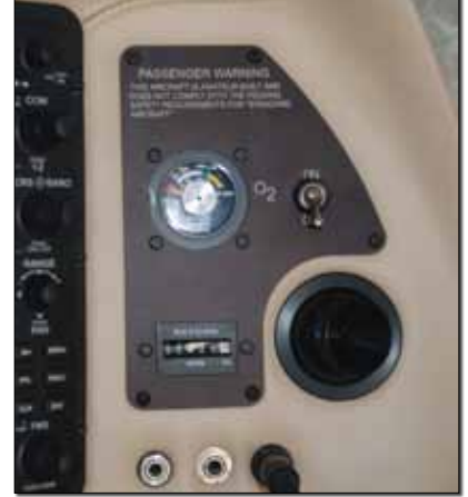
The oxygen meter and Hobbs meter fit nicely in this custom side panel by Evolution pro-builder Mike Custard.
