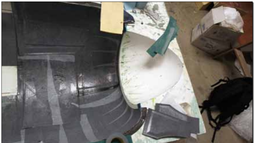
Notice how the soft tooling includes the spinner half.
