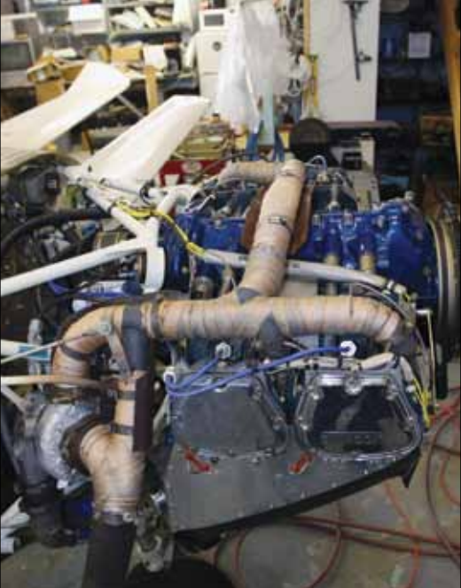
An uncommon updraft-cooled, top-exhaust Lycoming TO-360 powers the Catbird.
