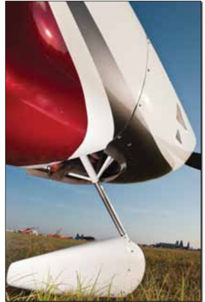
Arion has spent a lot of time getting the Jabiru to cool well. A substantial amount of cowling exit area and small lip help keep air flowing and temps down.
