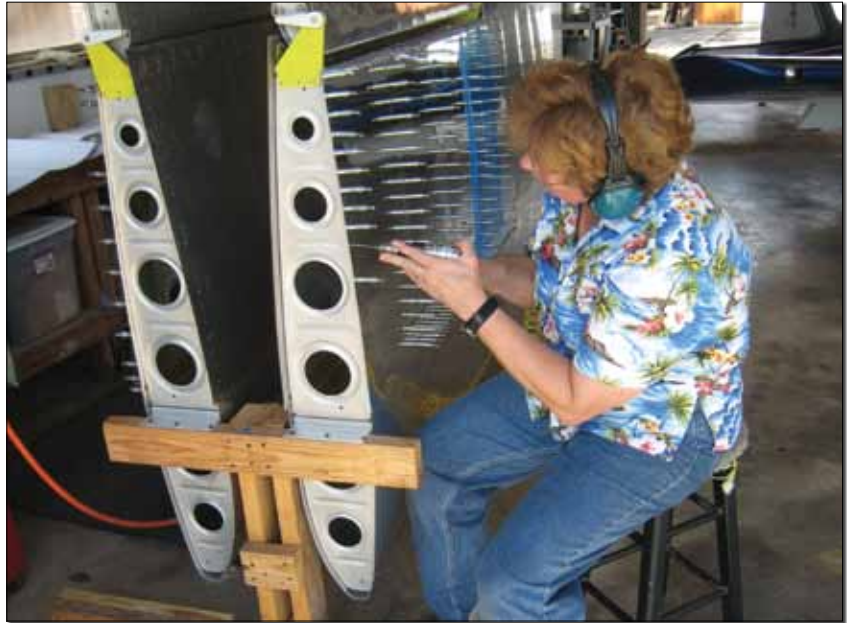
A well-designed aircraft has probably already had as many lightening holes as the creator considered prudent. These wingribs are a good example of the fact that it is hard to find additional material to remove safely.
