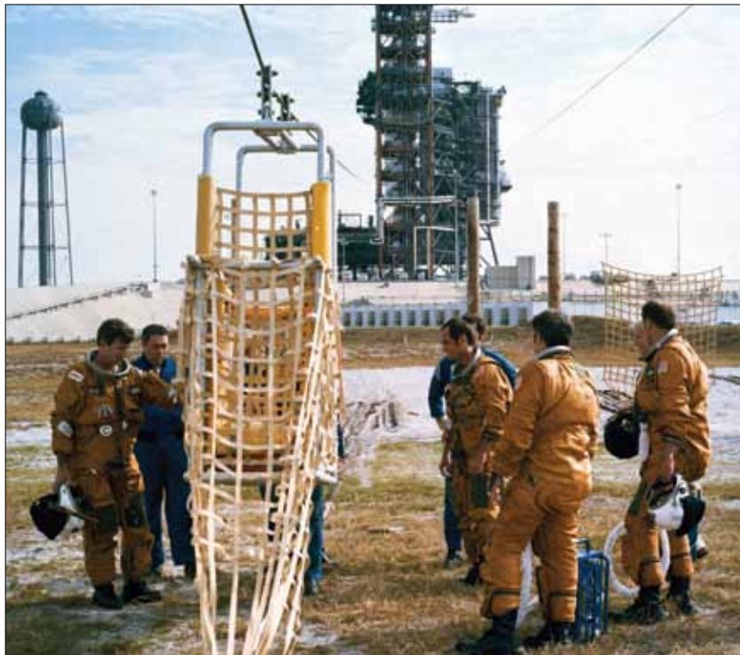
The Space Shuttle Launch Pad Escape baskets were an “E-ticket Ride” if there ever was one. Theory said they would whisk a person from the top to the bottom safely, but until they were tested, no one was sure. They were only tested with human occupants once, and that was enough.
