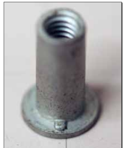
The anti-rotation key of a Rivnut can be seen here.
