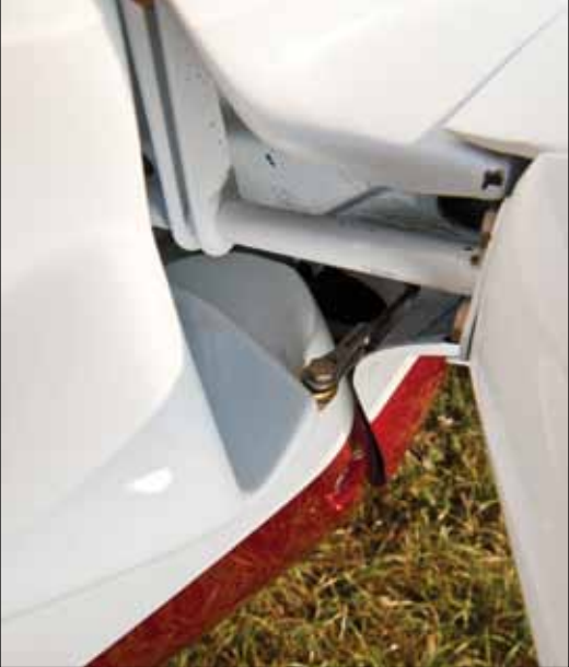
Traditional (for a homebuilt) flight controls include pushrod-activated elevator and ailerons, cable-motivated rudder.
