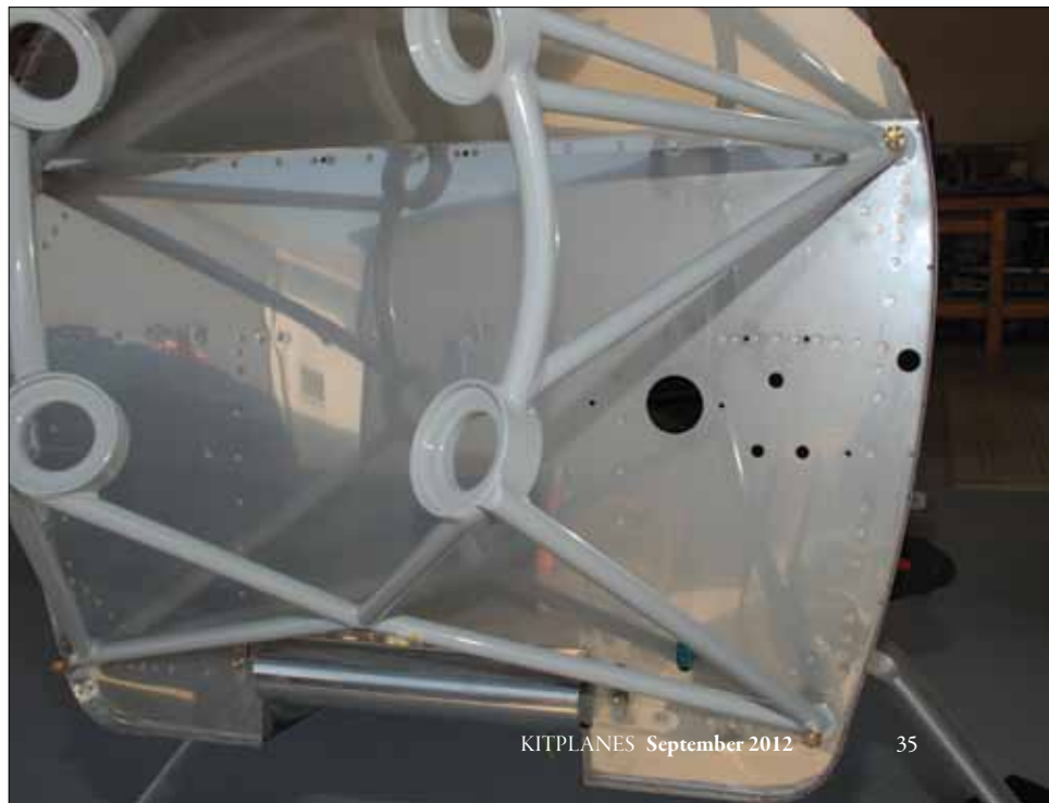
This RV-8 came with a prefabricated firewall with major holes already in place as part of the quickbuild option.
