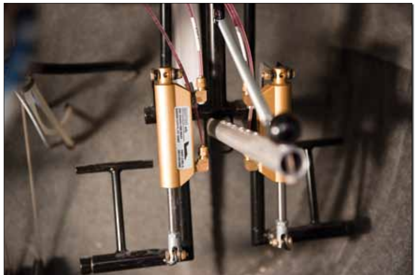
Because the seat does not adjust, the rudder pedals do. Note the small-diameter brake lines, which improve braking feel.
