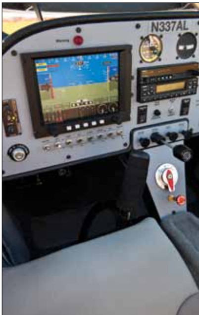
A GRT Avionics EFIS with synthetic vision and an integrated engine monitor anchor the Lightning's panel. Two seats are separated by a thin center console. A clever mixture adjuster (red knob) "fools" the Jabiru's Bing carburetor into reducing fuel flow in cruise.
