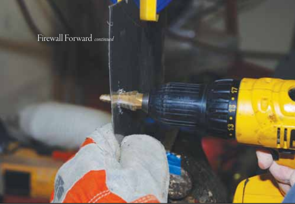
A step drill or Unibit makes easy work of drilling medium-size holes in sheet metal.
