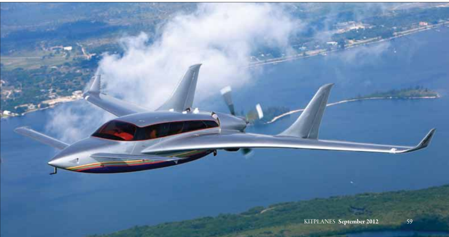
A dazzling image in flight, the Volaré shows off its twin vertical stabilizers.
