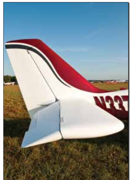
By adding 3 square feet of horizontal stabilizer, Arion's Nick Otterback gave the Lightning substantially improved pitch stability. The maximum throw of the top-hinged elevator was reduced 10° to 15° up. Electric pitch trim remains as a separate tab.
