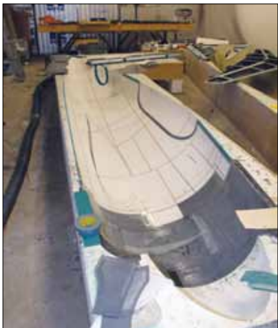
Soft tooling created by Sierra is used for the Stinemetz brothers' scale Bearcat.
