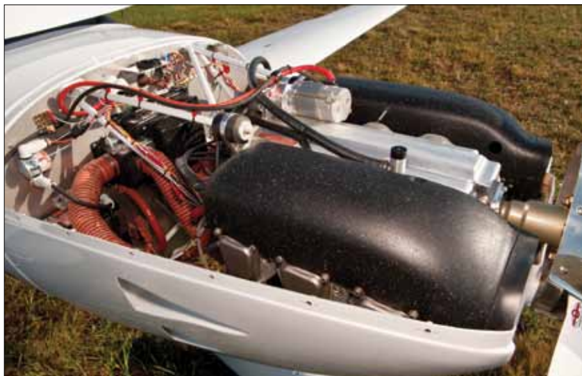
You can have any engine you want in the Lightning as long as it's the Jabiru 3300. This air-cooled, direct-drive engine makes 120 horsepower, just right for the airframe.
