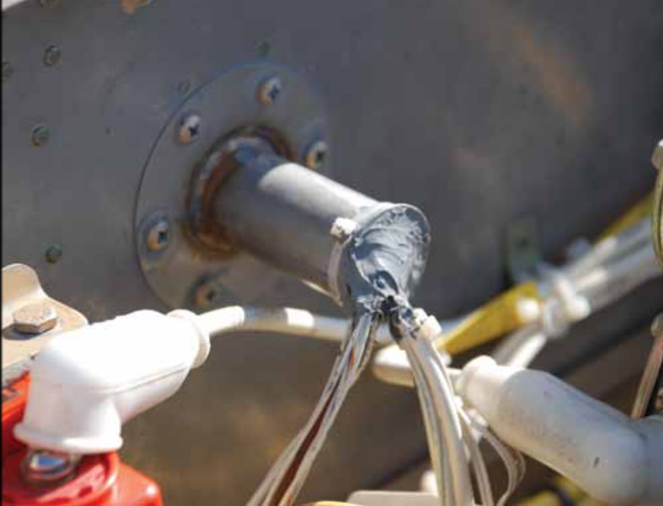
The Cessna factory uses a firewall tube filled with flame-resistant caulking for the wire penetration in the new 162 Skycatcher.
