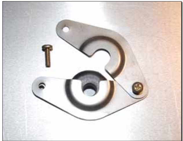
A firewall grommet shield is opened up to show the grommet. Wires with factory-applied connectors often need oversized holes in firewalls. The shield protects the grommet filling in the hole.
