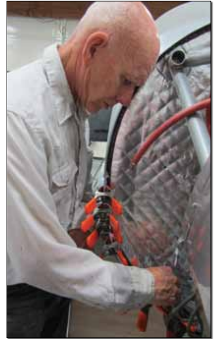
Wendell Solesbee works on the engine installation in his Lancair Evolution. Note the factory-furnished firewall blanket made to protect the composite structure of the airplane.
