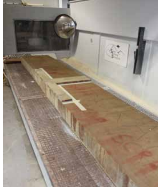
Sierra's milling machine makes quick work of large pieces of stiff foam for soft tooling.
