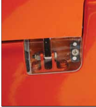
These acrylic aileron and flap hinge covers are one of the Solesbees' nice custom touches.
