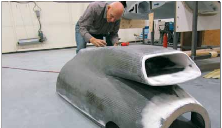
The engine cowl proved to be Wendell's greatest challenge, and that doesn't even consider the extra work of creating a blind fastener system for the cowl.
