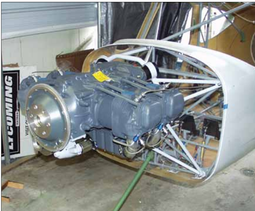
Here's a GlaStar under construction with a transparent firewall in place, ready to begin the process of positioning items on the firewall.
