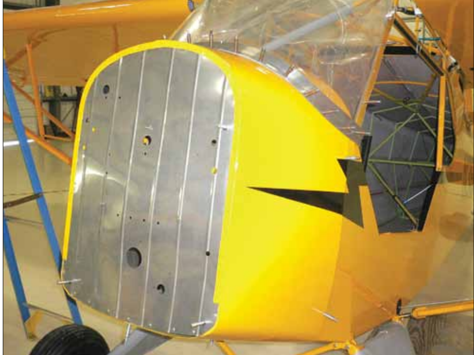
Ribs were rolled into this stainless-steel firewall to stiffen it up and prevent “oil canning.”
