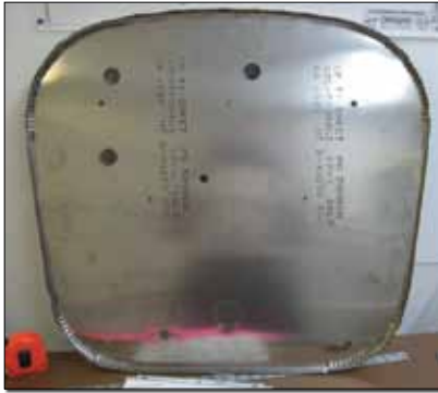
This Super Cub firewall by F. Atlee Dodge is made of commercial pure titanium and saves about 2 pounds compared to a stainless-steel firewall.
