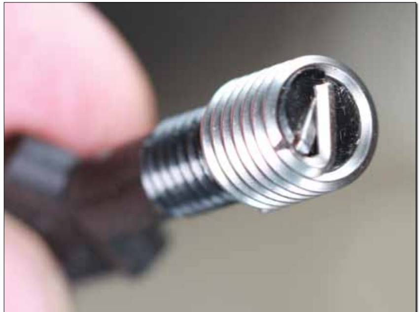
A Heli-Coil on the installation tool. After the coil is seated, the tang that catches the reinforced step of the tool is broken off and removed.
