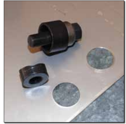
A chassis punch makes a much cleaner hole than a hole saw. Here are the two types of holes side by side, with the chassis punch hole being the lower one. Unfortunately, chassis punches cost considerably more than hole saws.
