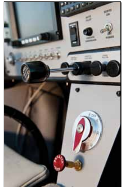
A GRT Avionics EFIS with synthetic vision and an integrated engine monitor anchor the Lightning's panel. Two seats are separated by a thin center console. A clever mixture adjuster (red knob) "fools" the Jabiru's Bing carburetor into reducing fuel flow in cruise.
