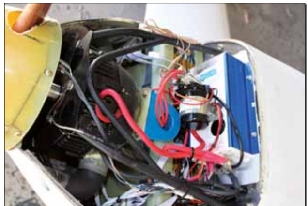
A compact electric motor and controller live under the Quickie's cowling.
