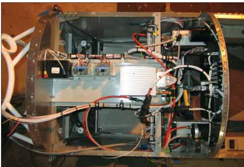
By contrast, here is the author’s RV-8, a very capable EFIS-equipped RV-8 completed seven years ago. The boxes are still modern, but they’re much larger than those produced today.
