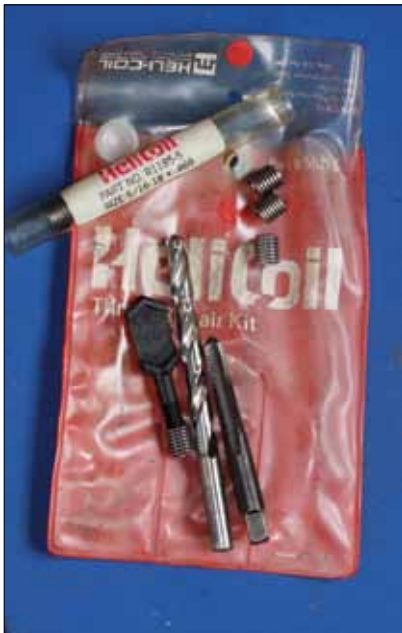
Heli-Coil kits contain an installation tool, a drill bit, and a special tap for cutting threads to receive the Heli-coil.
