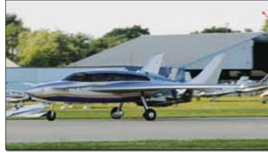
The Volaré can land and take off in 1500 feet, allowing use of various airports.
