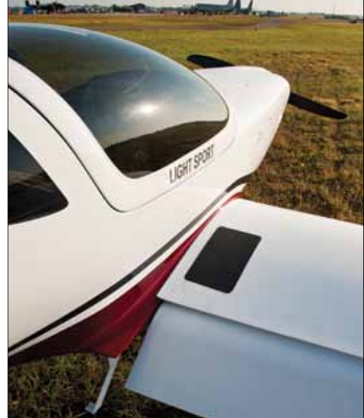
The wingroot fairing is part of the fuselage shell.
