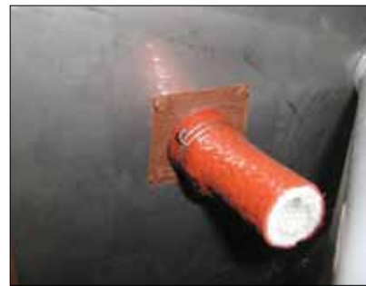
Glasair Aviation uses a stainless-steel sleeve with a piece of Aeroquip Fire-sleeve attached to route cables through the Sportsman firewall. After the cables or wires are run, the sleeve is filled with Flamesafe FS 1900 sealant.
