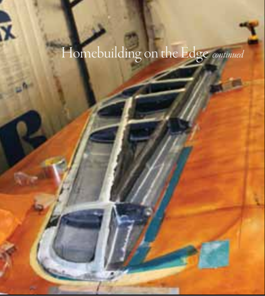
The Stinemetze Bearcat's horizontal stabilizer under construction in soft tooling.
