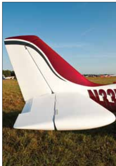
By adding 3 square feet of horizontal stabilizer, Arion's Nick Otterback gave the Lightning substantially improved pitch stability. The maximum throw of the top-hinged elevator was reduced 10° to 15° up. Electric pitch trim remains as a separate tab.
