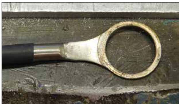
Figure 8: Purchased isolated junction thermocouple had poor thermal transfer characteristics.
