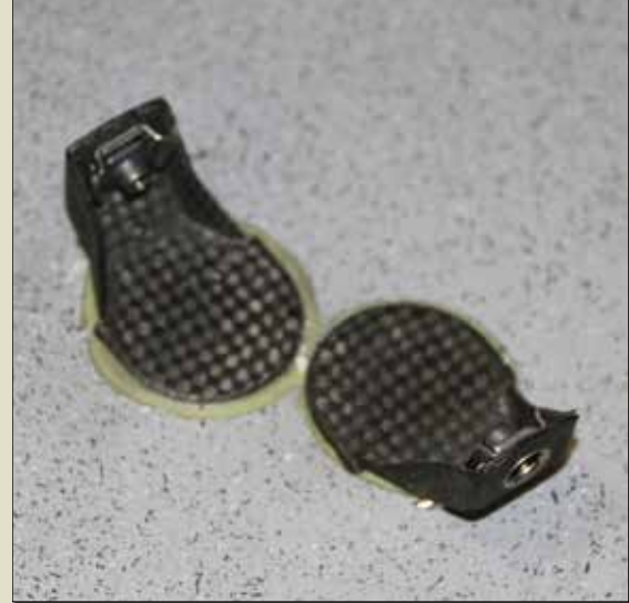
The "spoon" standoffs can be used to fasten wire bundles or, in this case, to serve as attachment points for a wiring tunnel cover.
