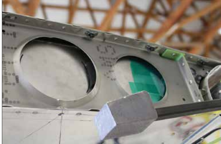
Click Bond has sold a wing tip attachment kit for several years for RVs. Here they did the same thing on their Sportsman.
