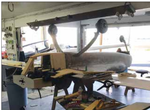
(Left) The original cowling on the “just overhaul the engine” VariEze was ridiculously heavy. To build the bottom cowling, we flipped the airplane upside down. (Right) Sometimes to work on the inside, it’s easier to put the fuselage on its side.
