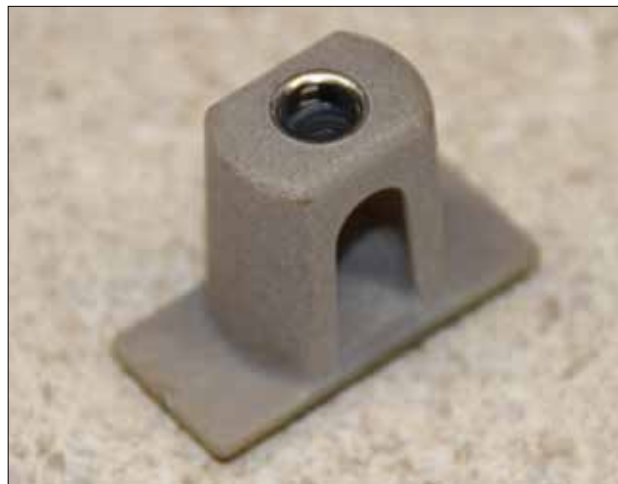
A standoff holds wiring bundles off of a floor or bulkhead to prevent chafing.
