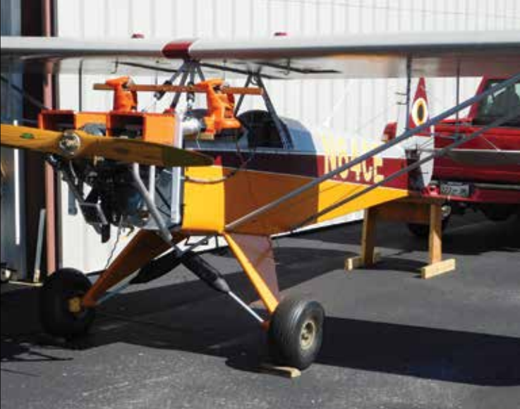
Figure 4: Front plenum covers off for pre-run check. Remember to set brakes on pickup truck.
