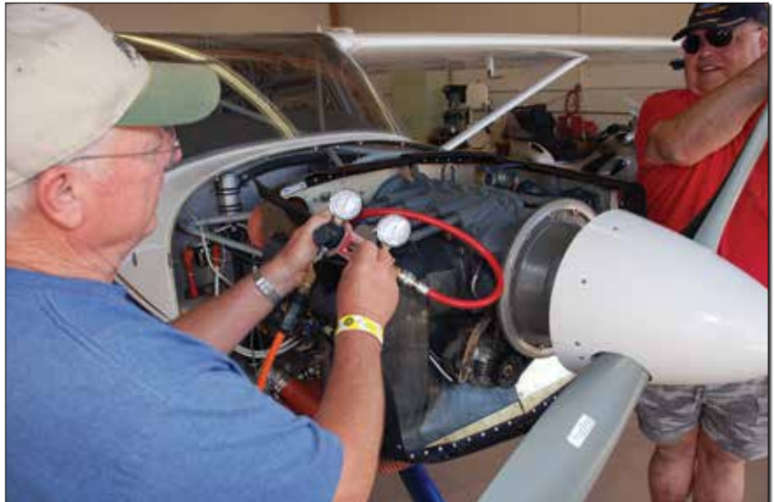
Longtime building buddy Ed Zaleski (left) performs a differential compression test on cylinder #1 while a friend hangs onto the prop to keep it from turning and injuring someone. The reference pressure will be on the left gauge, and the pressure in the cylinder will be on the right gauge.
