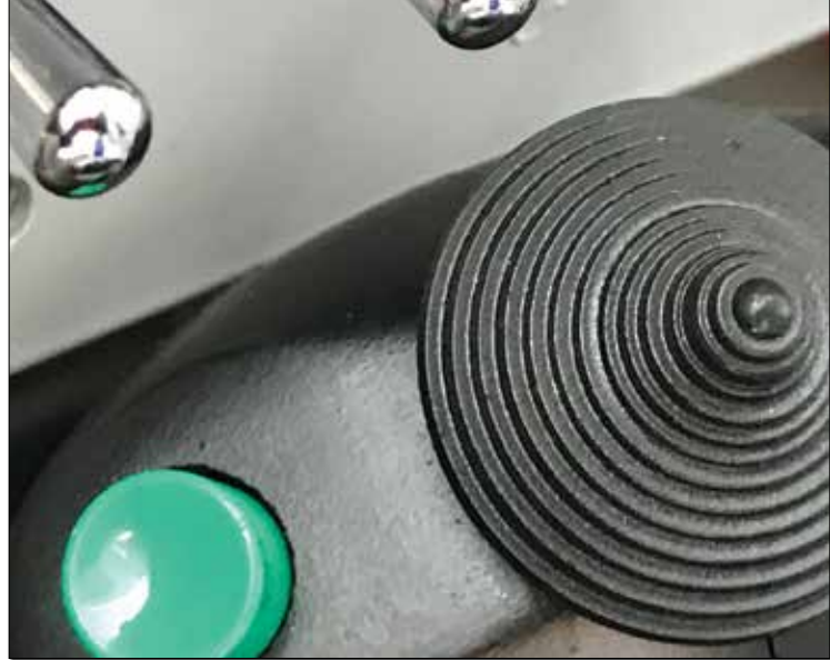
I see way too many examples of this: The stick hits the instrument panel and does not allow full forward control deflection.
