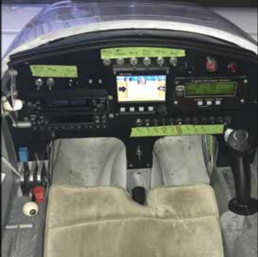
(Left) Even though snarky green tape with Sharpie ink is legal, you want appropriate placards on the panel. (Right) New mini EFIS and audio panel installed in a Long-EZ.
