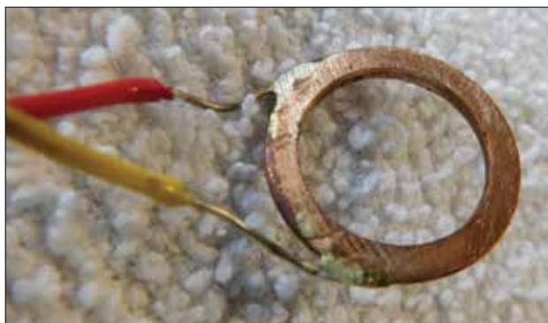
Figure 9: Homemade washer thermocouple (resting on terry cloth towel) gave accurate readings.
