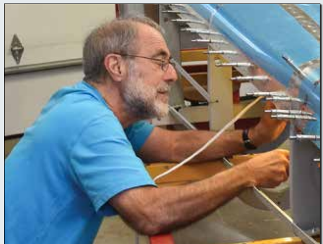
David Paule rivets the left-hand skin of his RV-3B. He finds building to be both fun and challenging, and he haven't gotten bored yet.
