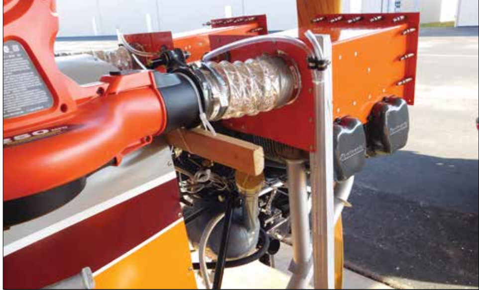
Figure 3: Aero engine with addition of forced air cooling for ground running.
