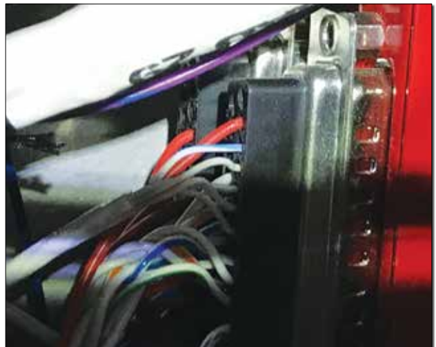
D connectors require a backshell that provides strain relief for the wiring, as well as screws for fastening them to the device. Do not leave them off like pictured here!
