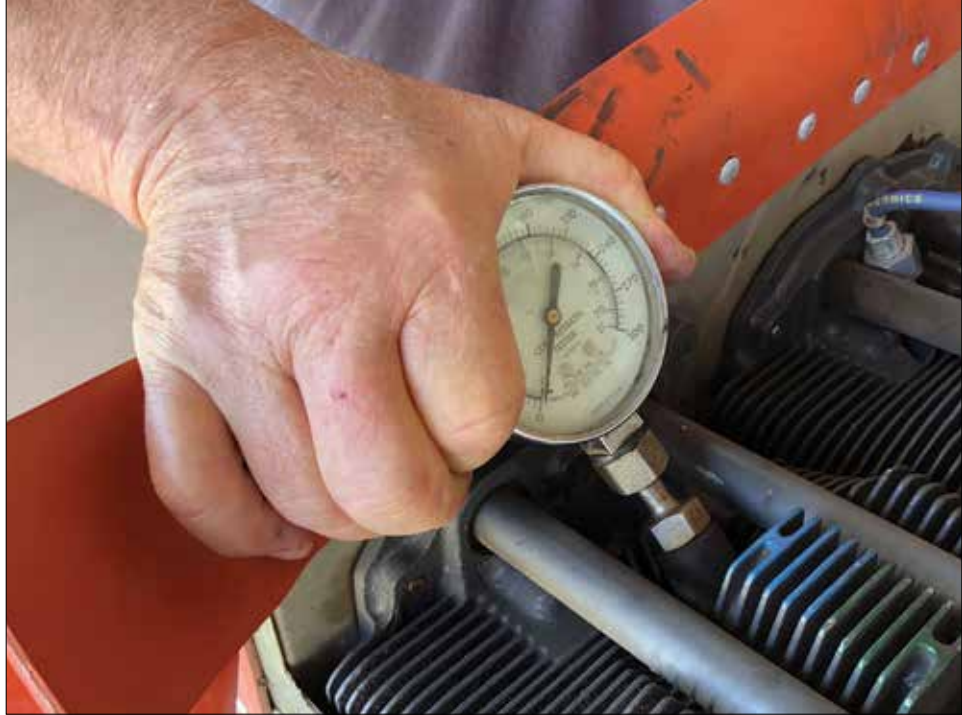
An automotive-type compression tester can be used as an alternative means of checking cylinder condition if that is all that is available. This is not a substitute for a proper differential compression tester, but it can provide some useful information.
