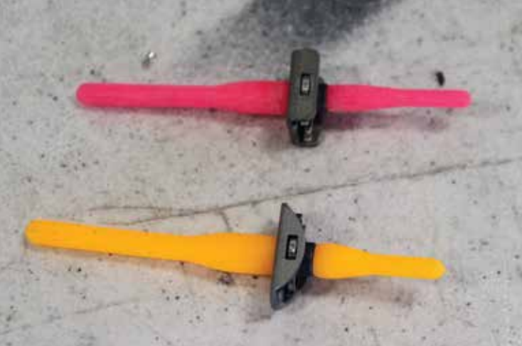
Nut plates come in standard sizes—here is a compact #6 and a standard #8. The different color fixtures tell you the size.
