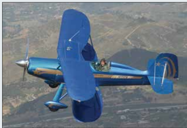
Tom flies his Starduster Too over north San Diego County, California. With its O-540 Lycoming, it climbs at 2500 fpm, cruises at 150 mph, and has a 350-foot takeoff roll.
