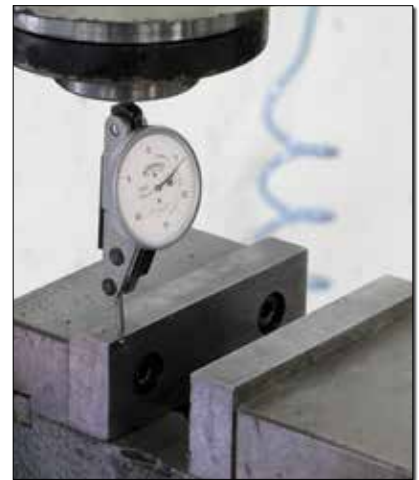
Using a test indicator to square a vise. Note the dial reading "suggests" the left side is about 0.005-inch forward of the right side.
