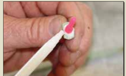
Apply the adhesive to the nut plate all around the fixture.
