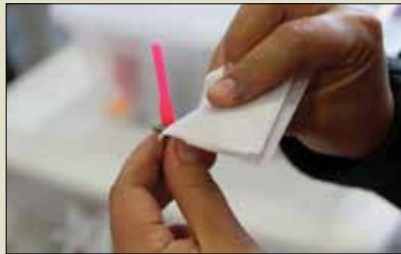
Use the Click Bond cleaning wipes to clean both the nut plate and the surface to which it will be applied.
