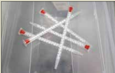
The disposable tips for the gun have spiral mixing inserts so that the adhesive is ready to cure when it exits the tip.
