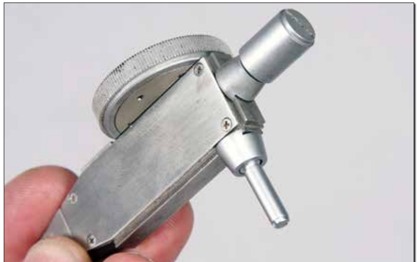
This test indicator has dovetail rails on the top and back for fixing compatible mounting posts.
