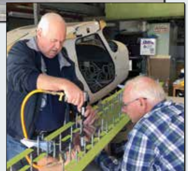
Dave Prizio (left) and Ed Zaleski assemble a Sportsman flap for their new GlaStar project. The Sportsman flaps should be an improvement over the original GlaStar flaps, but require extra effort to make them work. Dave's first GlaStar is shown above.
