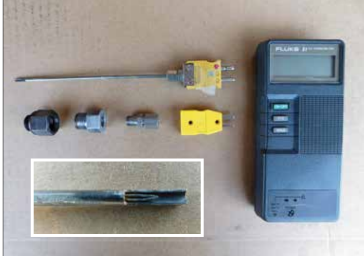
Figure 7: Exposed junction type-K thermocouple (inset) and handheld thermocouple readout used to accurately read oil temperature.
