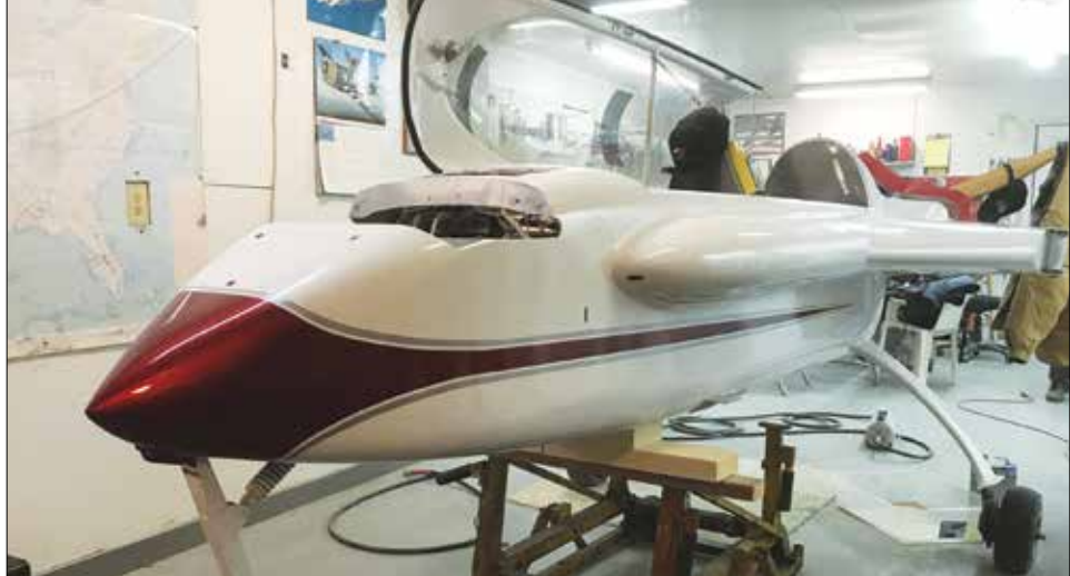
(Left) What's an engine overhaul without new baffling? A really good job on baffles is a 10-day process. (Right) The red and silver are House of Kolor paints that require a clear coat.
