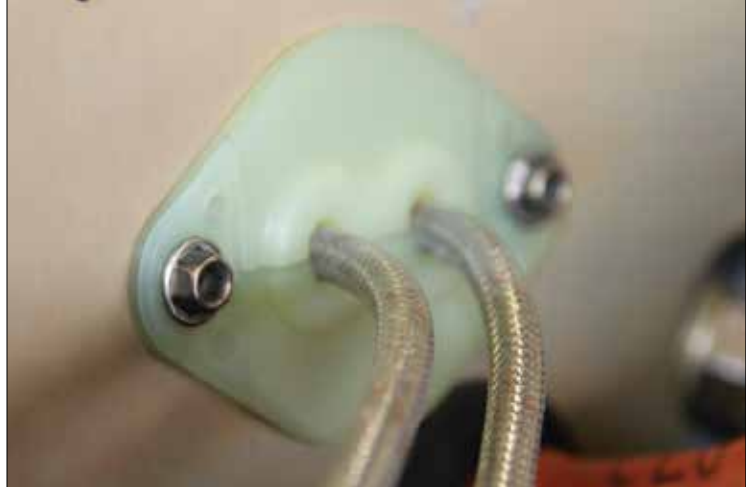
Here, the hollow Click Bond screws are used with nut plates to hold spark plug baffle grommets in place.
