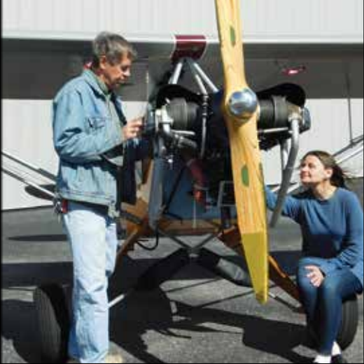
Michael Leigh and Beate Ellis check the A-75 engine for leaks and loose components, which often try to ruin a sunny day.
