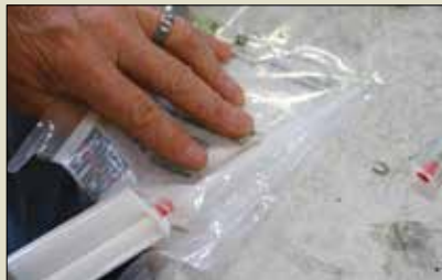
If you have let the gun sit with adhesive in the tip for a few minutes, clean it out by squirting the semi-cured adhesive into a waste plastic bag until you get the nice white color.
