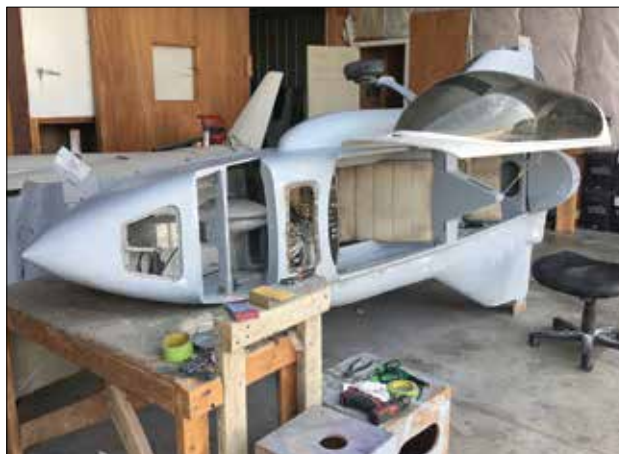
(Left) The original cowling on the “just overhaul the engine” VariEze was ridiculously heavy. To build the bottom cowling, we flipped the airplane upside down. (Right) Sometimes to work on the inside, it’s easier to put the fuselage on its side.
