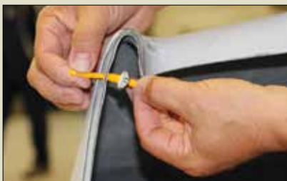
Thread the fixture through the hole to pull the nut plate up to the surface.
