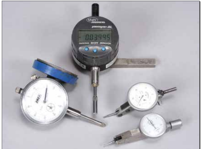
Dial and digital indicators (left and top) can't be beat for precision linear measurement. But for squaring up mill vises, “dialing in” lathe parts (aka adjusting concentricity), dial test indicators (right) are the workhorses of the machine shop.
