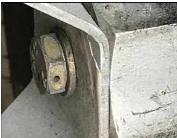
Drilled head bolts are drilled for a reason. Usually the part is subject to high vibration or rotation, such as this wheel pant bracket. It requires safety wire. I pointed this out to one builder/pilot and received a very questioning look. I was vindicated when we looked at the other wheel pant and the bolt was completely missing!
