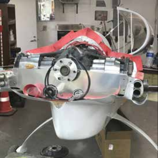
(Left) What's an engine overhaul without new baffling? A really good job on baffles is a 10-day process. (Right) The red and silver are House of Kolor paints that require a clear coat.
