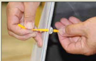
Pull the fixture until you hear a little pop, and the nut plate is seated fully.
