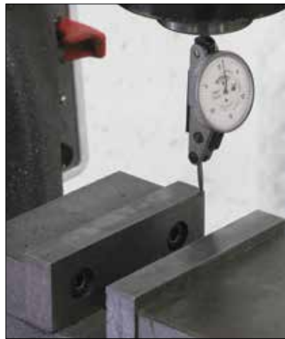
Using a test indicator to square a vise. Note the dial reading "suggests" the left side is about 0.005-inch forward of the right side.
