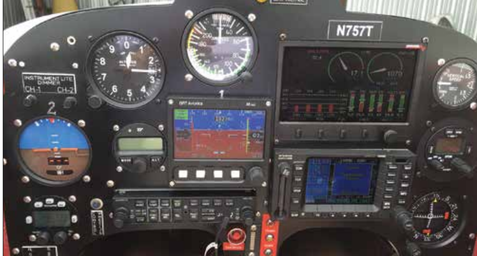
(Left) Even though snarky green tape with Sharpie ink is legal, you want appropriate placards on the panel. (Right) New mini EFIS and audio panel installed in a Long-EZ.
