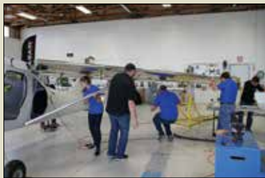
Students help to fold the wing on the Sportsman in preparation for installing fuel lines.
