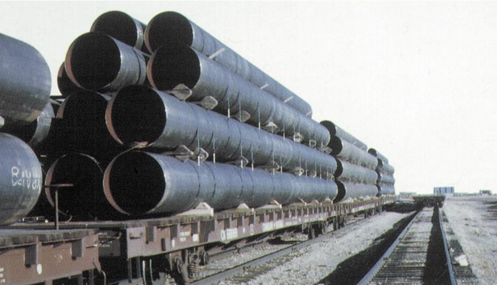
Delivered to the Foothills gas pipeline expansion project in Canada, these 42-inch diameter steel pipes expanded the Foothills system to a total of 606 miles of pipeline as of November 1, 1998.
