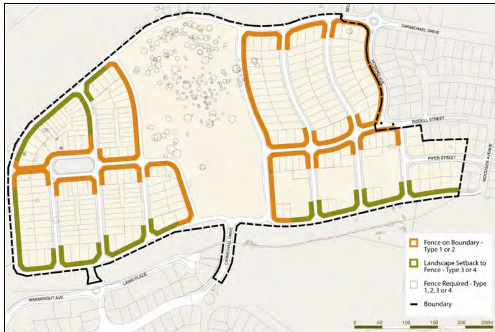
Figure 13 Fence Type and Location
