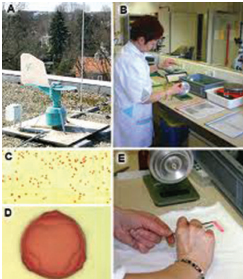
Figure 2 Pollen and mold assessment: A: pollen trap; B and E: ELISA measurement; C and D: microscopic evaluation of pollens and molds.
