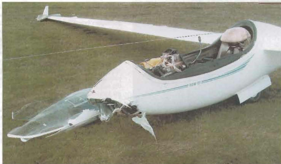
Modern brittle composites, such as carbon fibre resins used in sailplane structure, have greatly increased static strength. On the other hand, research indicates inadequate performance on dynamic impact
