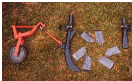
Lay out of coulters system. (right to left) front fertiliser tube, slot cutting blades, seed delivery, press wheel
