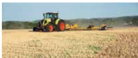
This 15m Claydon Straw Harrow is used immediately after harvest to encourage volunteers and weed seeds to germinate, allowing them to be controlled cheaply and effectively before the next crops is drilled.
