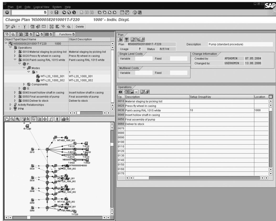
Figure 4.11 "Production Process Model" Transaction in SAP APO, Transaction /SAPAPO/SCC03
