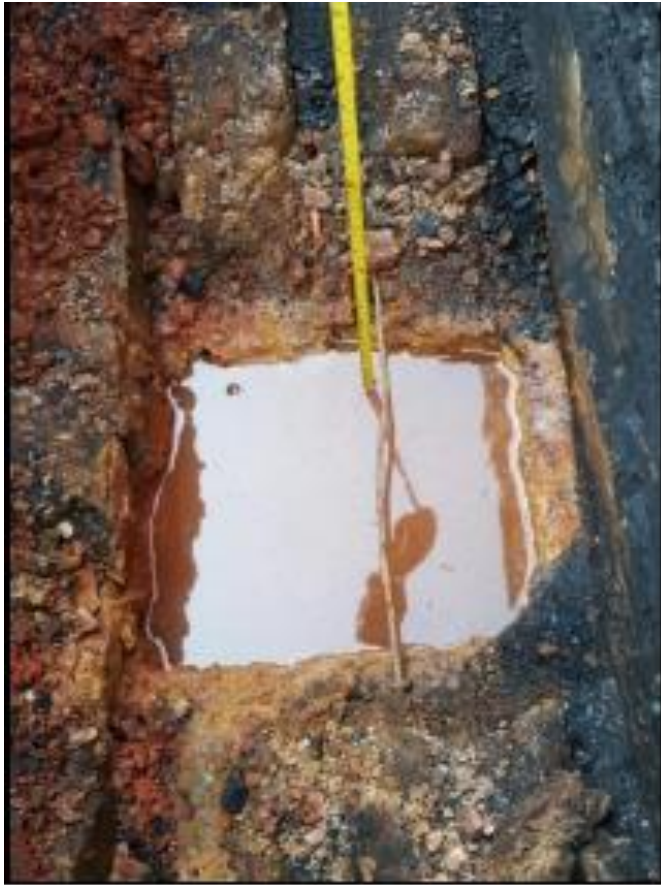
Figure 35: Falling head permeability test setup.
