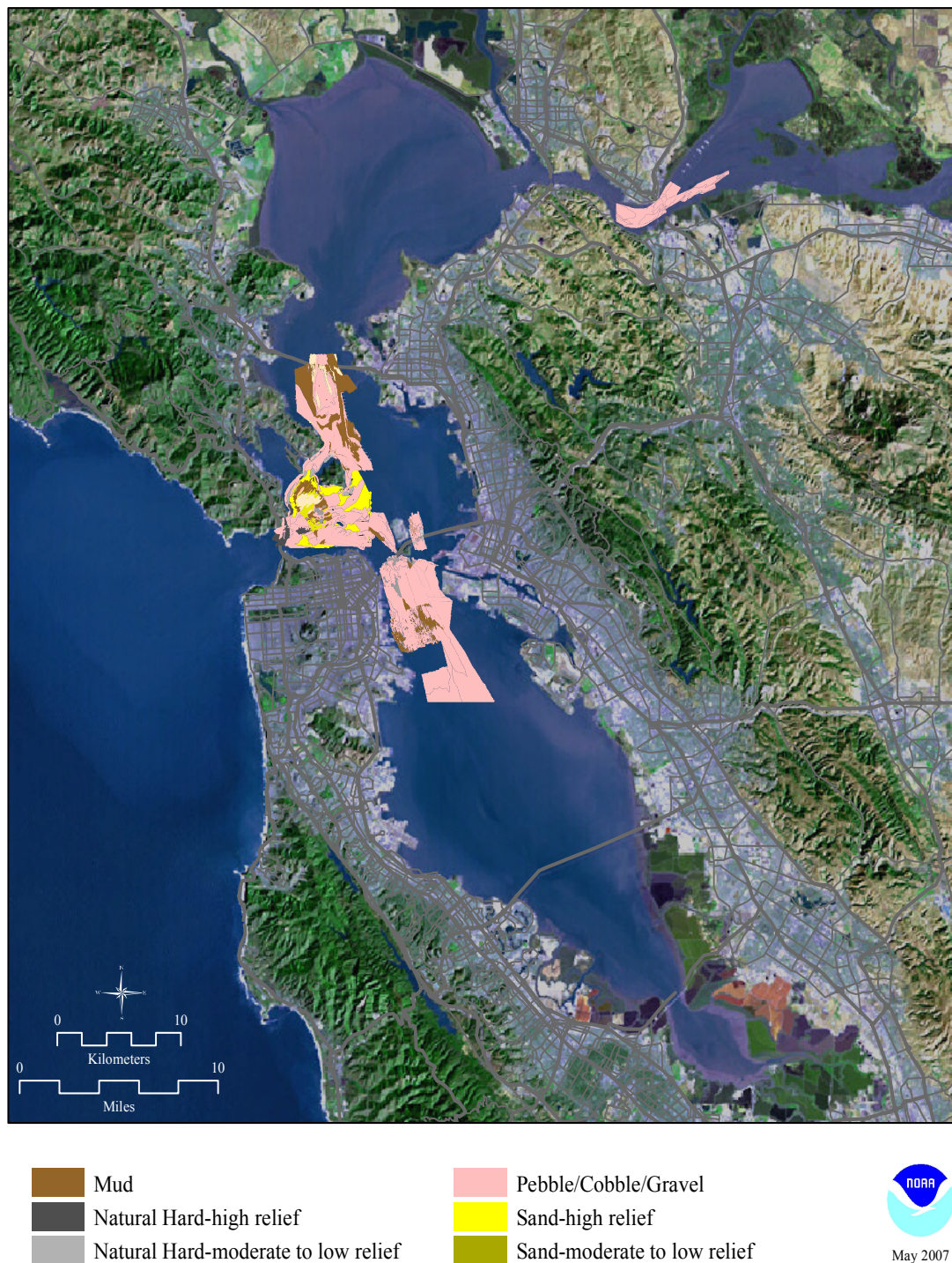
Figure 10. Soft bottom and hard bottom substrates in San Francisco Bay interpreted from multibeam bathymetric images and side-scan sonar mosaics after Greene and Bizarro (2003).
