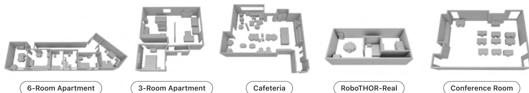
Figure 3.2: Examples of environment templates for our five target test environments. These are produced by an iPhone scanning each environment using our iOS app that leverages Apple’s RoomPlan API. These environment templates contain the room layouts and some 3D locations for large furniture objects. They do not contain small objects, textures, lighting, etc.
