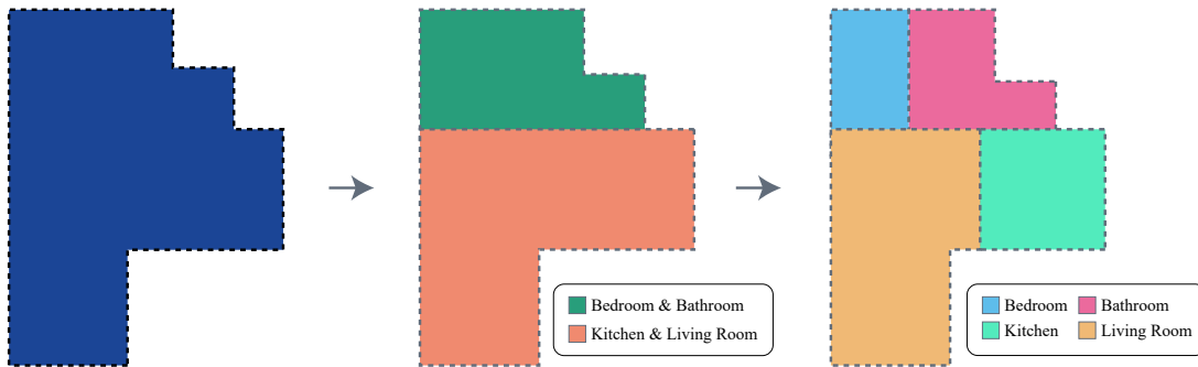
Figure A.9: An example of the recursive floor plan generation algorithm, given an interior boundary and the room spec in Figure A.6a. Here, we first divide the room into a “bedroom & bathroom” and a “kitchen & living room” zone. Then, within the “bedroom & bathroom” zone we place both the bedroom and bathroom, and within the “kitchen & living room” zone, we place both the kitchen and living room.
