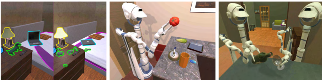
Figure 1.8: Interactivity. Object states can change ( e.g. , the laptop or the lamp in the left panel), and the agents can interact with objects and other agents (middle and right panels).
