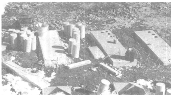
Figure 6. Tests also involved taking cores, casting cylinders, and making thermocouple measurements.
