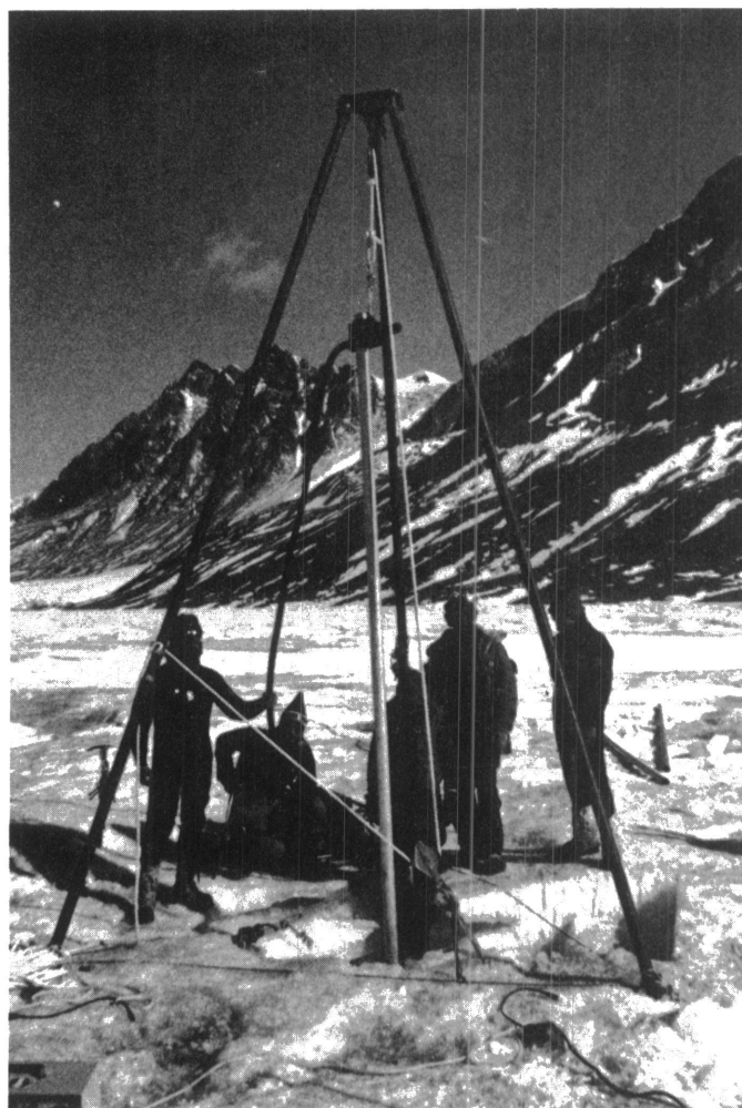
Vibracore operation on Lake Hoare. The vibracorer consists of a Wyco electric vibrator connected to a 20-foot section of aluminum pipe. The vibrator is powered by a high-cycle generator.
