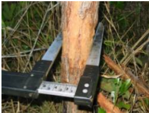
Figure 42: Use of precision calipers
