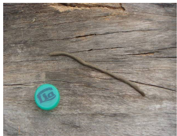
Figure 7: Field technique demonstrating the presence of clay in the soil (>50%).
