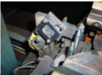
Fig. 9 — Unprotected plastic-bodied photoelectric sensors don't stand a chance in weld cells.
