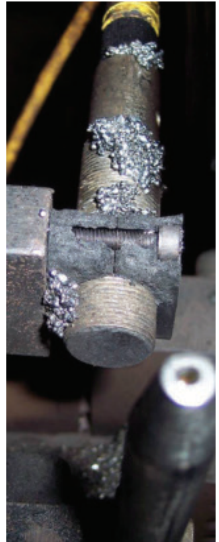
Fig. 7 — These plastic brackets have been eaten away by slag and heat.
