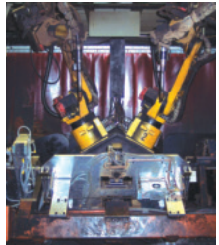
Fig. 12 — This well protected weld cell is ready for months of maintenance-free operation.
