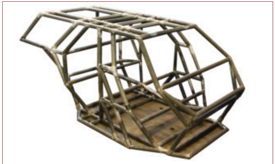
Fig. 5 — EWI concept tubular space frame incorporating magnetic pulse welding, deformation resistance welding, and controlled short circuit gas metal arc welding technologies (Al-steel).
