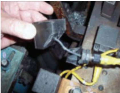
Fig. 3 — A sensor destroyed by impact.
