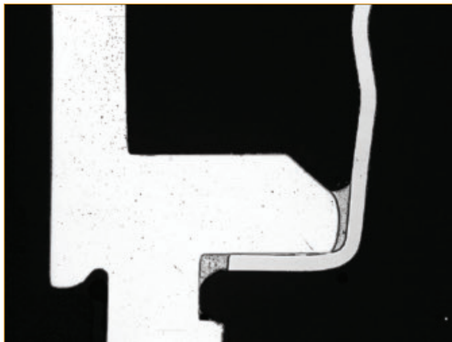
Complex lap joint made with Sn-Sb solder for a high-reliability assembly.
