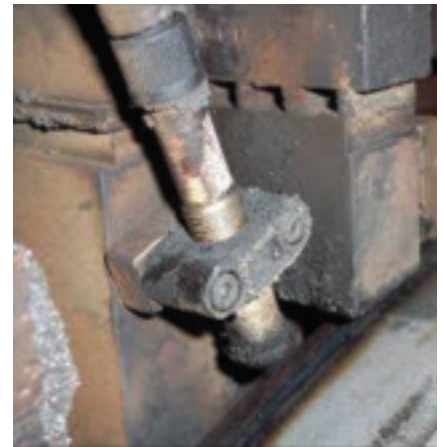
Fig. 1 — A sensor being destroyed by heat and slag.
