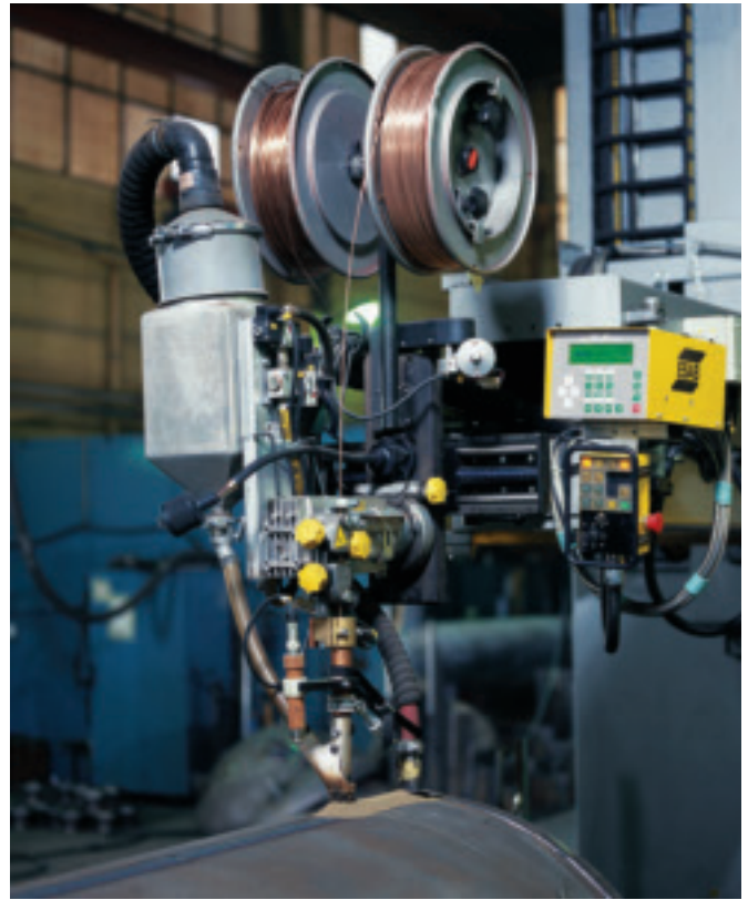
Many of the fluxes used in subarc welding applications, such as the one shown here, will be produced at ESAB's latest flux plant.
