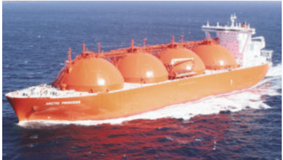
Fig. 1 — Liquid natural gas (LNG) tanker with four large welded aluminum spheres (tanks).
