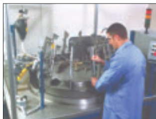
Rotary Index Machine 400 parts per hour
