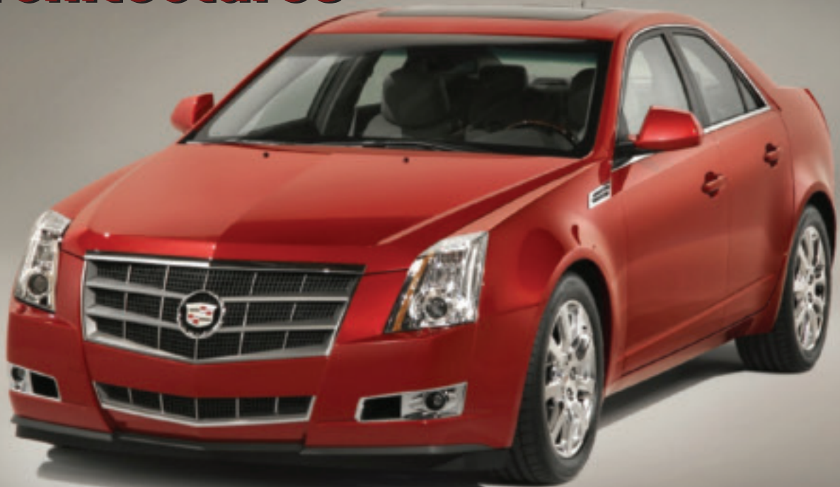
The Cadillac CTS features an aluminum hood. (Photo courtesy of Novelins.)
