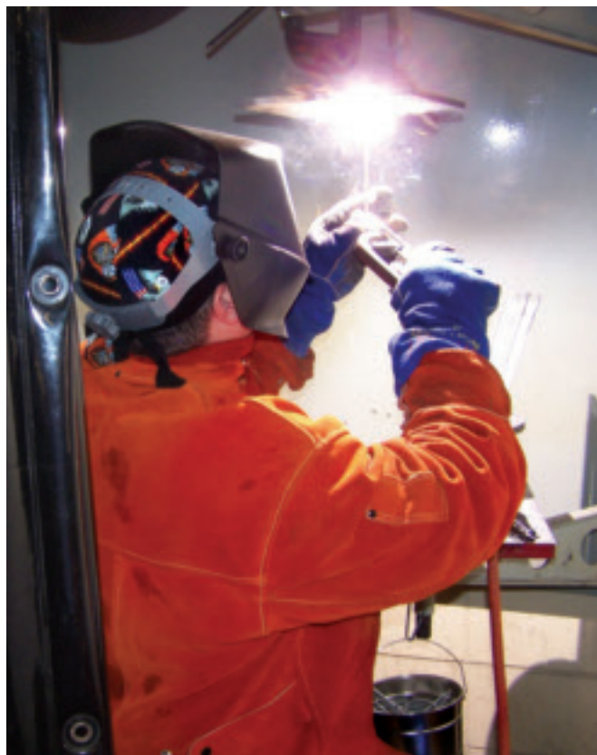
Student Joe Wright works on his overhead plate test using shielded metal arc welding.
