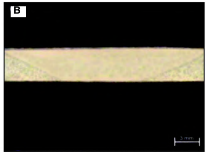
Fig. 2 — Optical macrographs showing the stirred zones (SZ) of the 63/37 brass joints obtained at a rotational speed of 1600 rev/min. Traverse speeds are as follows: A — 175 mm/min; B — 200 mm/min. The plate thickness is 3 mm.
