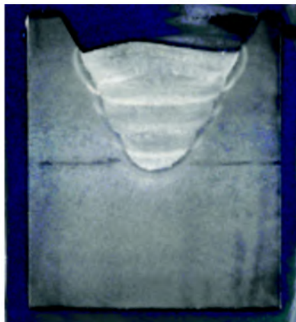
Fig. 2 — A 1-in.-deep groove weld created using T-GMAW in the vertical (3G) position with upward progression.
