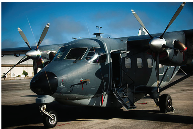
The C-145A Skytruck is a light cargo and troop transport aircraft designed and manufactured for the US Air Force (USAF). The aircraft is primarily used to assist Aviation Foreign Internal Defence (AvFID) missions of the Air Force Special Operations Command (AFSOC). The transport aircraft can be reconfigured to perform precision combat airdrop, combat search-and-rescue, humanitarian assistance, casualty evacuation and disaster relief missions. Originally brought into the AFSOC inventory in 2009 as M-28 Skytrucks, the C-145A has remained continuously deployed since March 2011. (U.S. Air Force Photo).
