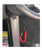
Figure 2-6. Emergency Engine Stop Switch
