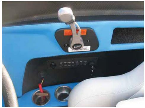
Figure 2-2. Circuit Breaker Panels
