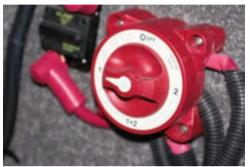
Figure 4-8. Battery Switch
