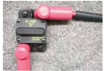
Figure 4-12. Main Circuit Breaker
