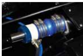
Figure 4-6. Drip Less Shaft Packing
