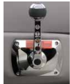
Figure 2-20. Throttle Control for Boats Equipped with Electric Shift
