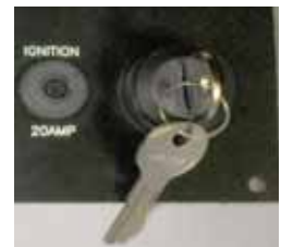
Figure 2-15. Remote Ignition Key Switch
