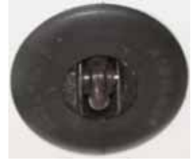
Figure 2-37. Thru-Hull Paddle Wheel Pickup
