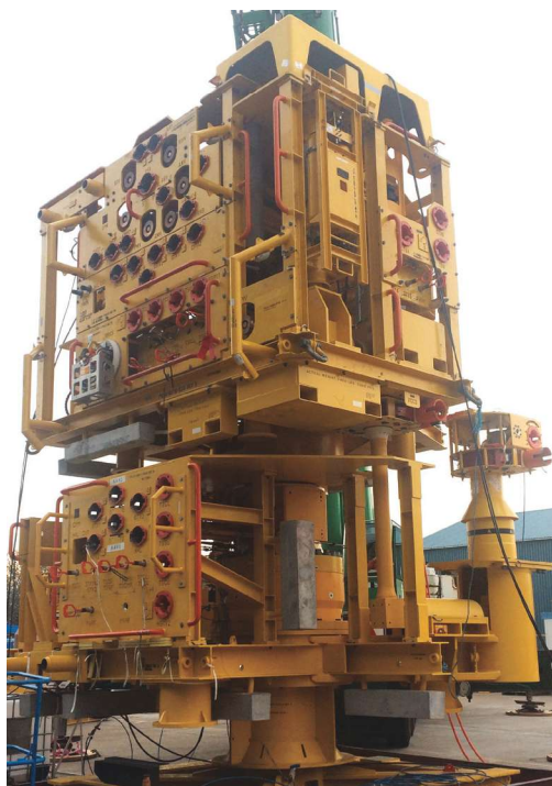
The DVXT, a deepwater vertical tree, benefits from a modular approach to engineering and manufacturing, with application engineers able to focus on designing customization where it is needed. (Source: Baker Hughes, a GE company)
