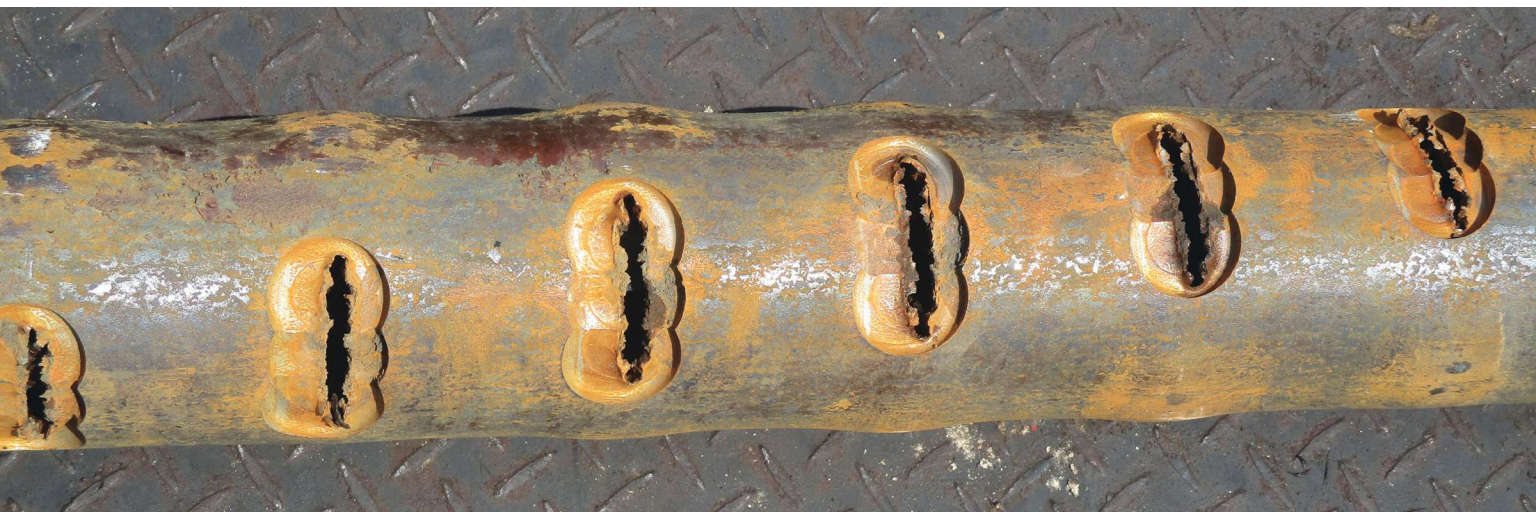
FIGURE 1. The perforations cover all voids and microannuli between the casing and formation or within the cement. (All images courtesy of DynaEnergetics)
