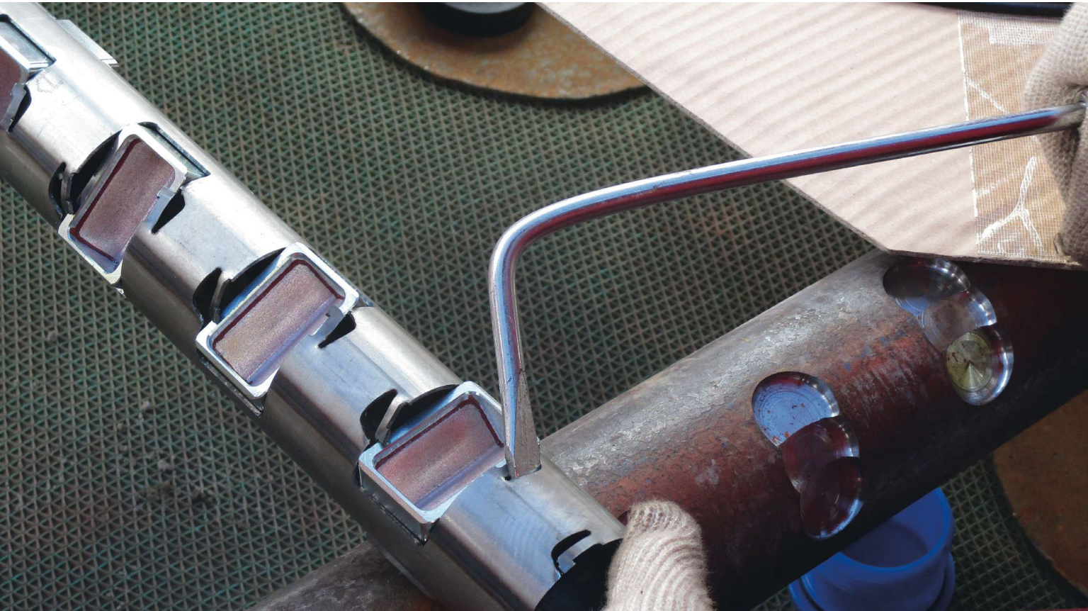
FIGURE 2. The slot gun design produces a helical pattern of horizontal rectangular slots in the tubing to achieve 360-degree access to the area behind the tubing or casing.
