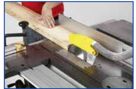
Circular saw with sliding carriage and side mitre fence Sierra circular con escuadradora e guía lateral
