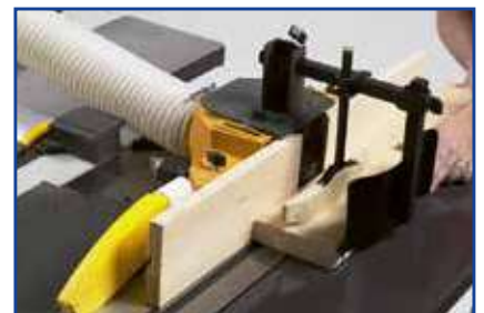
Spindle moulder for contour working and joints construction and wood assembling.
