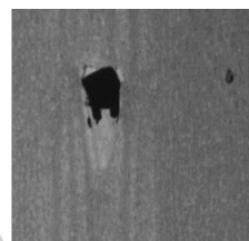
Holes detected at the winder can be traced back to locate the source and root cause of the defect.
