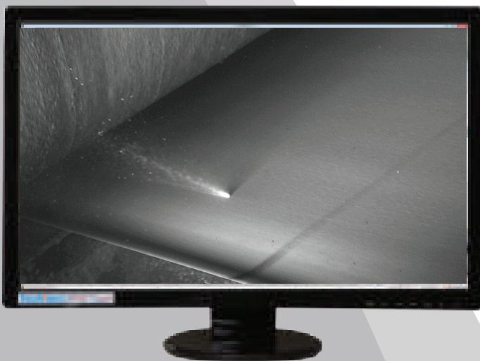
Dirt on the sheet captured by WebVision cameras could be the cause of a break further down the line.
