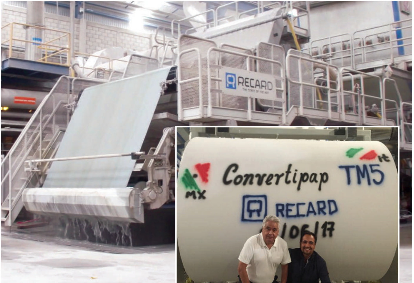
Above: Convertipap's most recent TM started-up in June 2017 and increased the company's production capacity by 25,000tpy;
