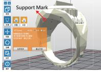
Manual editing: you may add or delete support structure based on the features of the print manually. To add support, simply select a proper size of the contact point and then click on the model at the top of where support is required downward. To delete support, just click on the support mark (the blue dot). After setting up support marks, click "Generate" to continue.
