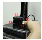
Finally tighten the screws with a coin or other tools (sequence from F1, B1, F2 to B2) and press [OK] to complete calibration.
