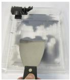
② Scrape off the residue stuck on the tank gently. Avoid damaging the silicon finish.
