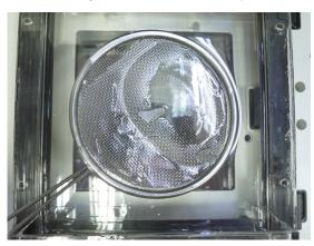
② Mop the fingerprint or resin under the tank or on the glass with with lint-free cloth dampened with alcohol.
