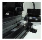
Wait for 5 seconds so the silicon finish on the tank can reshape. Check the tank frame has repositioned (there's no gap between the frame holders).
