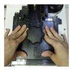
When you see the message above, press the platform with both hands 3 times. Make sure you see the right side of the tank sinks into the tank slot slightly.
