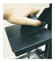
① Remove the platform Wear gloves before removing the prints. Turn the platform locker counterclockwise until it stops. And pull the platform to remove it.
