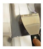
① Pour uncured resin in the tank into a waste bin. For remaining resin, scrape the surface of the tank gently while pouring the liquid out.
