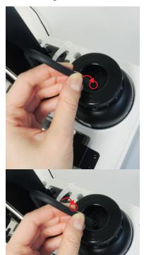
①Push the tubes all the way down. First attach the black tube to thick nozzle, and then connect the transparent tube to thin nozzle.
