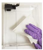
⑤ You can either wait until the alcohol in the tank evaporates completely or wipe away the alcohol with a lint-free cloth.
