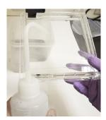
④ Spray alcohol on the tank and the silicon finish, and wait for around 1 minute. Gently scrape residue and pour remaining alcohol left in the tank into the waste bin. Repeat these steps until all residue has been removed.
