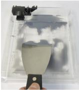
④ Cleanup and reinstall Remove any residue in the resin tank. Operate gently to avoid scratching the surface of the resin tank. Reinstall the resin tank after cleaning.
