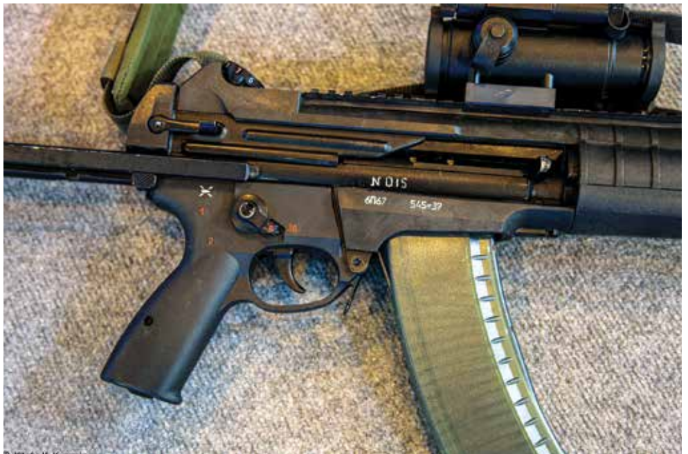
Early version of the A-545 rifle; close-up view of firing controls.
