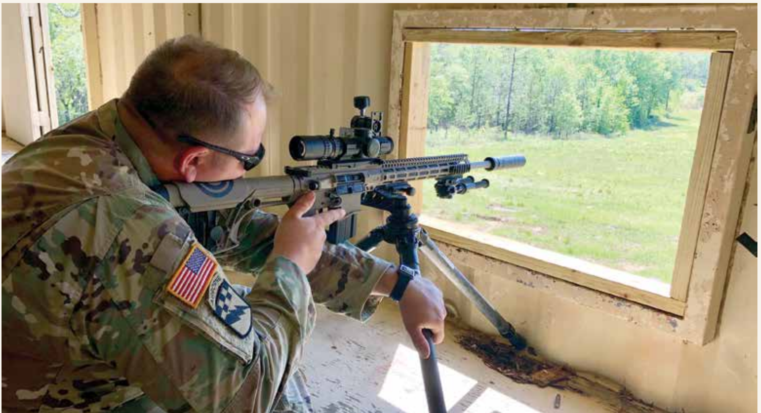
Utilizing tripod systems like this CruXord setup can help maximize stability when firing from alternate positions.
