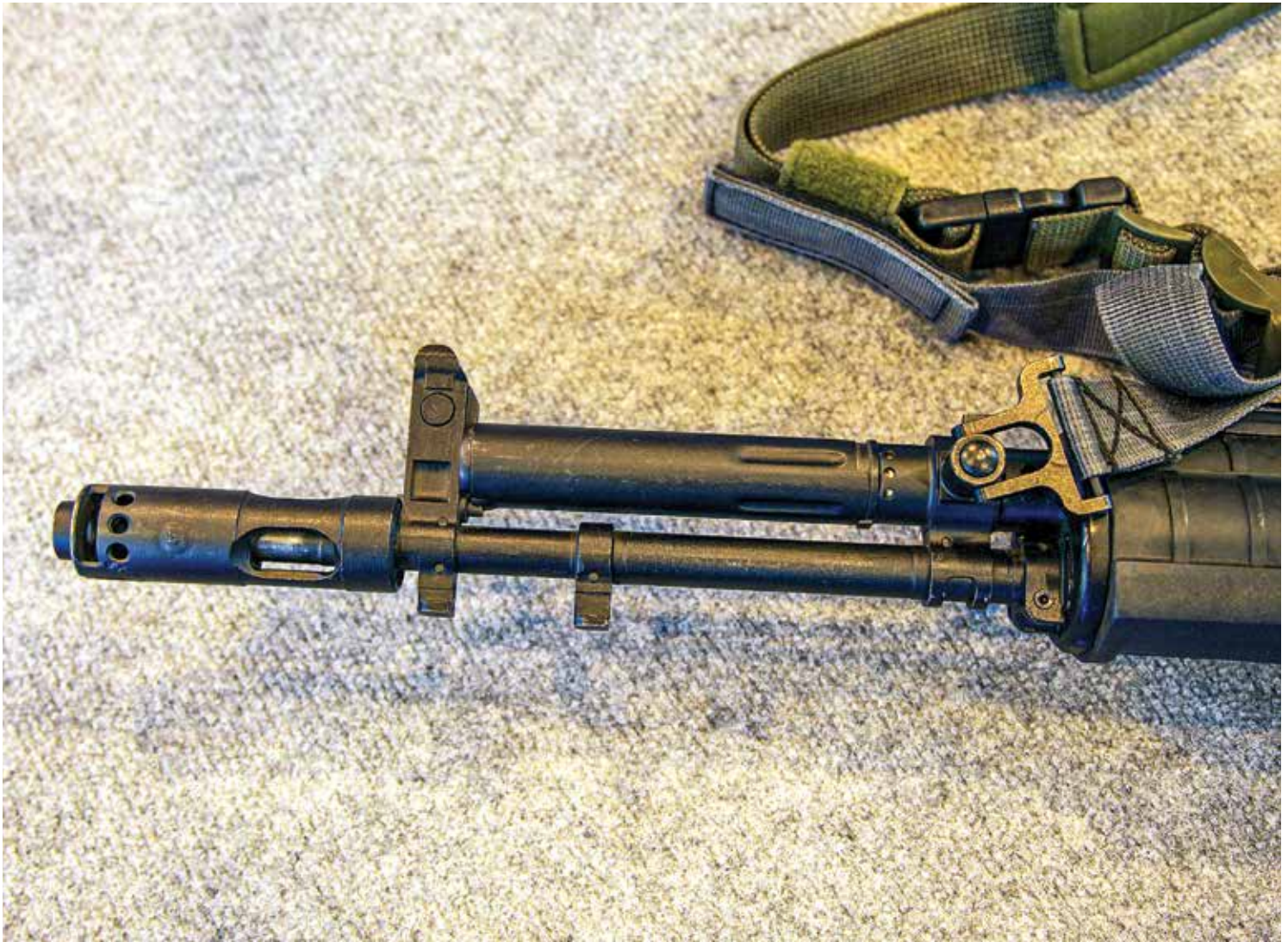
An earlier A-545 rifle, muzzle end and forward gas cylinder for balancing piece.
