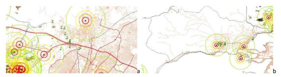
**Fig. 4.** Buffer zones of 500, 1000, 1500 and 3000m for SEVESO type industries, for municipality of Fyli – Ano Liosia (a) and for Municipality of Megara – Nea Peramos (b).
