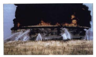
Figure 3. External cooling of tank walls in a full surface fire (HM Fire Service Inspectorate 2000)
