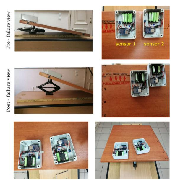
Figure 2. Pre-failure (upper part) against post-failure (middle part ) view for sensor 1 and sensor 2. Invalid experiments view (lower part), showing composite sliding.
