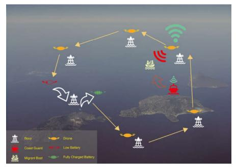
Figure 3. Visual description of the Automated Network for Air-Sea Actions: Each buoy charges one UAV per time. The aerial surveillance is divided into 2 sets. The UAVs of each set are activated simultaneously and move to their following buoy (clockwise order). When a set is operating, the UAVS of the other set are recharging. This loop continues throughout the day and provides a 24/7 surveillance.
