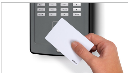
Time registration with RFID card
