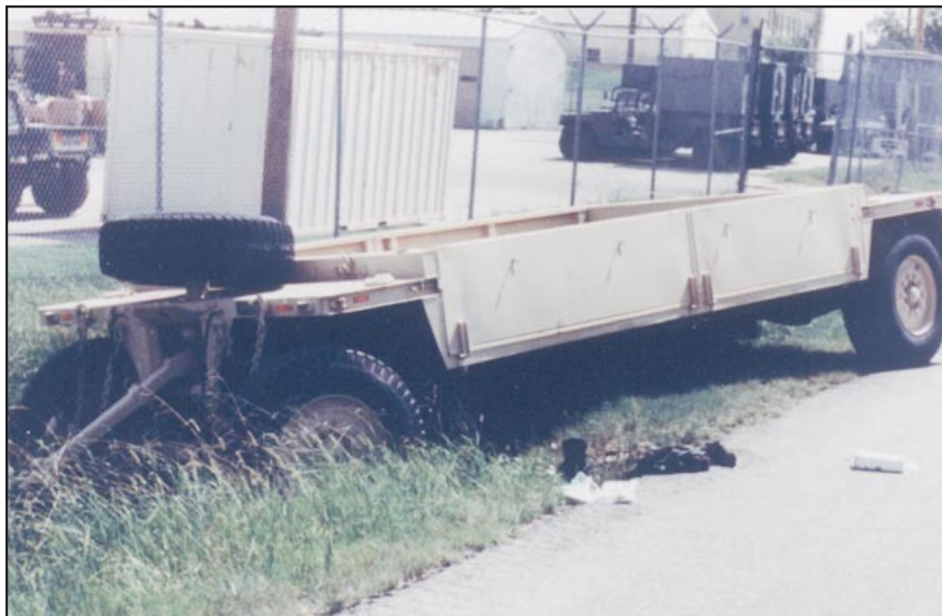
A soldier was killed when this trailer rolled over him while he was attempting to steer it away from parked vehicles. The risk assessment did not cover all aspects of the operation, and controls were not in place that could have prevented this accident.
