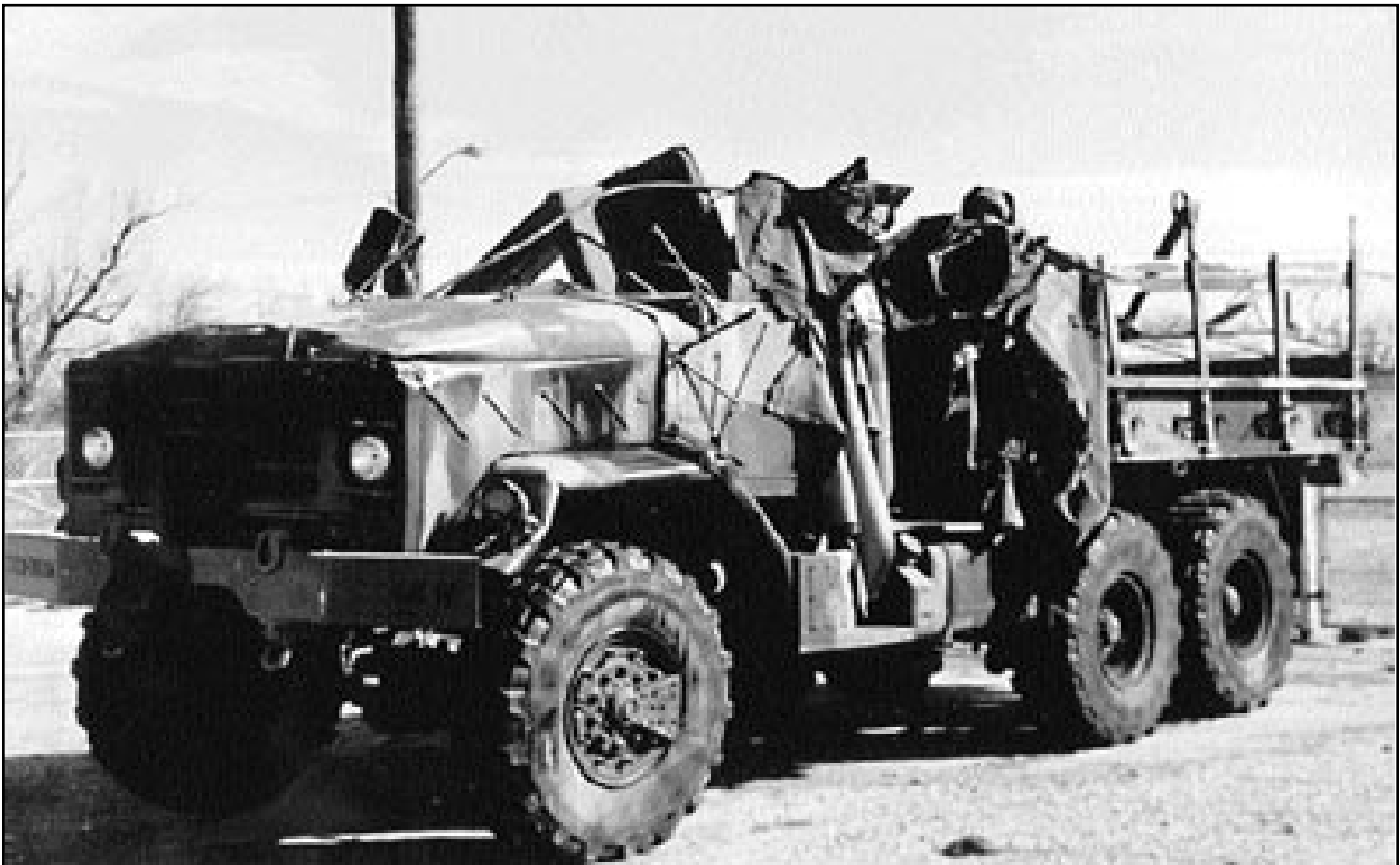
This M923A2 5-ton overturned while attempting to negotiate a curve at 45 MPH. The two passengers were killed.
