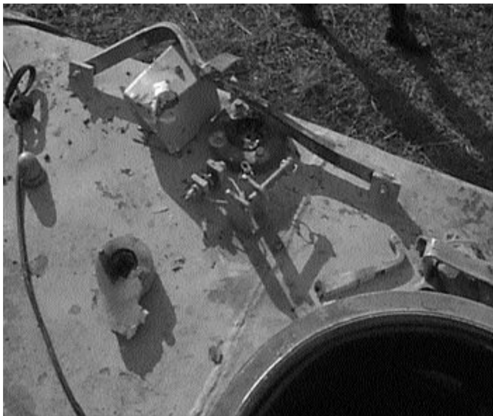
The M113 driver was killed when the M1A1's gun tube struck his vehicle, tearing off the driver's hatch
