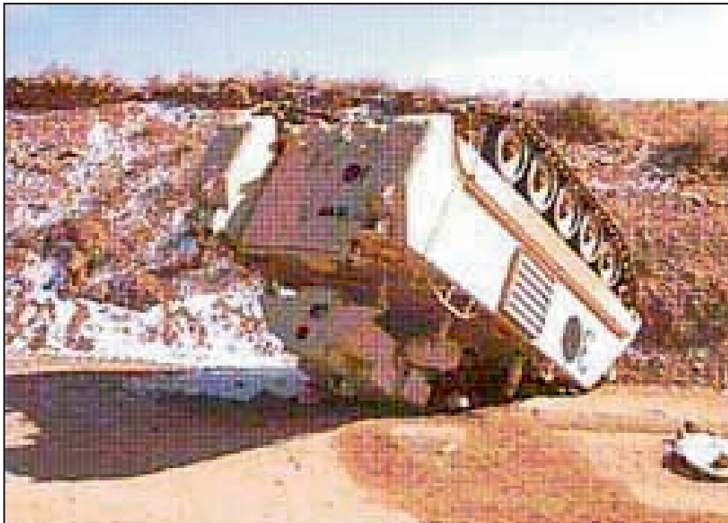
The driver of this M981 lost control as the vehicle was descending a 7° slope, turned to the left and ran upon an embankment. The vehicle overturned resulting in one fatality, three soldiers injured and vehicle damage.
