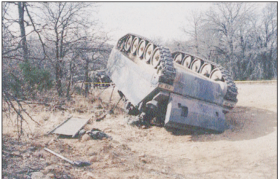
An improperly adjusted left lateral resulted in this FISTV making a sharper left turn than expected when the driver applied normal pressure. This and the vehicle's speed caused it to vault through the air and overturn.
