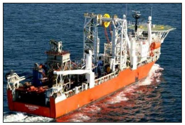
Figure 6: Example of a dedicated drill sampling vessel
