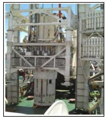
Figure 15: Example of the 2.5 m diameter drill bit within the drill frame structure
