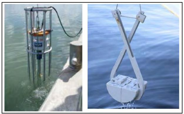
Figure 12: Left Example of a corer and right a Van Veen grab that works like a claw to grab sediment from the seafloor
