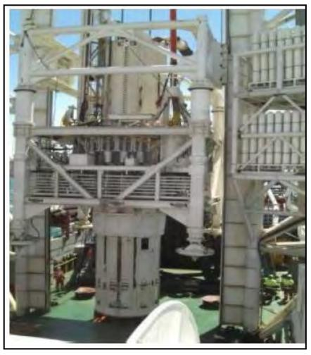
Figure 7: Example of the 2.5 m diameter drill bit within the drill frame structure
