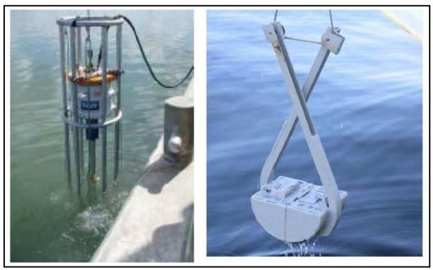
Figure 5: Left Example of a corer and right a Van Veen grab that works like a claw to grab sediment from the seafloor
