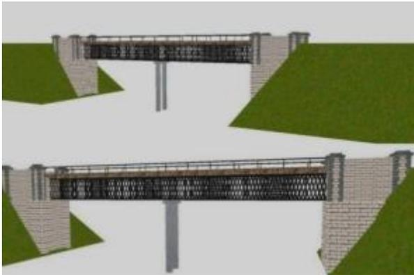
Figure 6.32: Example of lattice type structures that will allow for corridor continuity.
