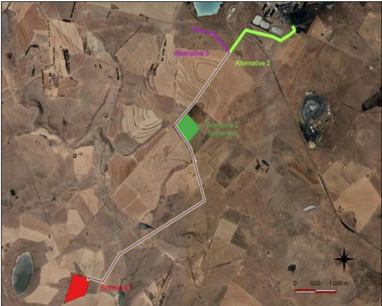
Figure 8: Pipeline alternatives for Ammonia 1.
