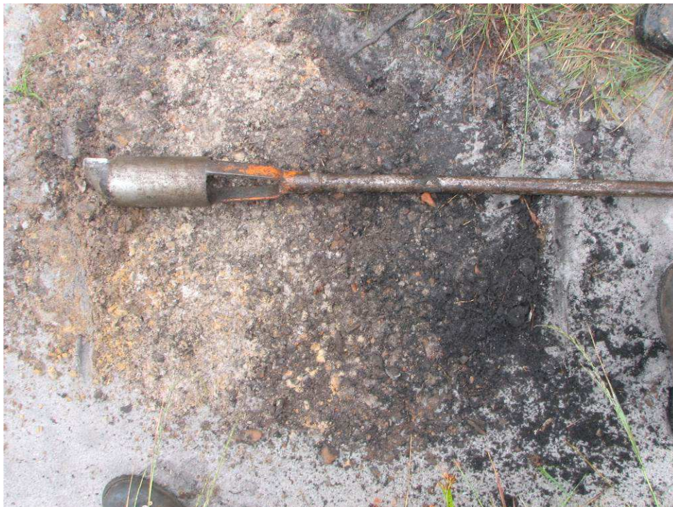
Photograph 1: Augered Cartref soil form with three distinct horizons displayed, including lithocutanic on the left, lighter coloured E-horizon in centre and an organic rich orthic A horizon towards the right
