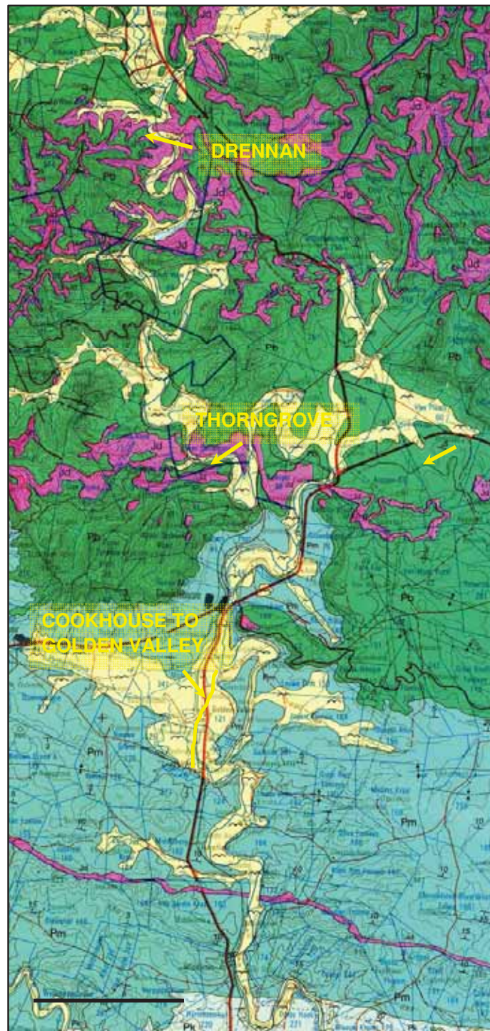
Fig. 4. Extract from 1: 250 000 geology map 3224 Graaff-Reinet (Council for Geoscience, Pretoria) showing location of the proposed loop extensions at Drennan, Thorngrove (both underlain by the Balfour Formation, Pb) and Cookhouse – Golden Valley (underlain by alluvium and the Middleton Formation). See Table 3 for summary of geology and fossils within rock units along this section of the Transnet manganese ore export railway line. Scale bar here = c. 10 km.
