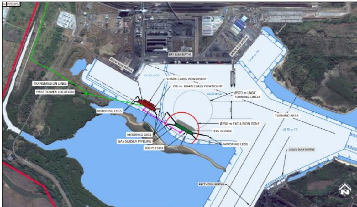
Figure 9-2 Alternative 2 for the position of the powerships.
