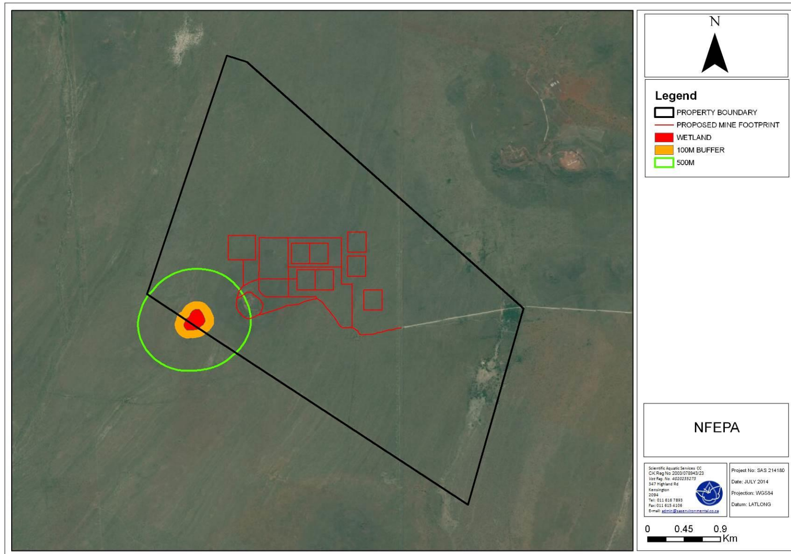
Figure 8: Natural wetland pan as delineated on site with associated 100m buffer and an indication of the 500m radius surrounding the pan.
