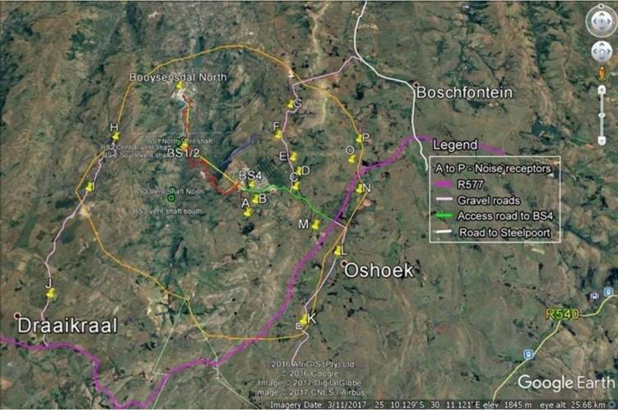
Figure 10-7 Noise, Vibration and Air Overpressure Receptors (Source: dBAcoustics, 2018)
