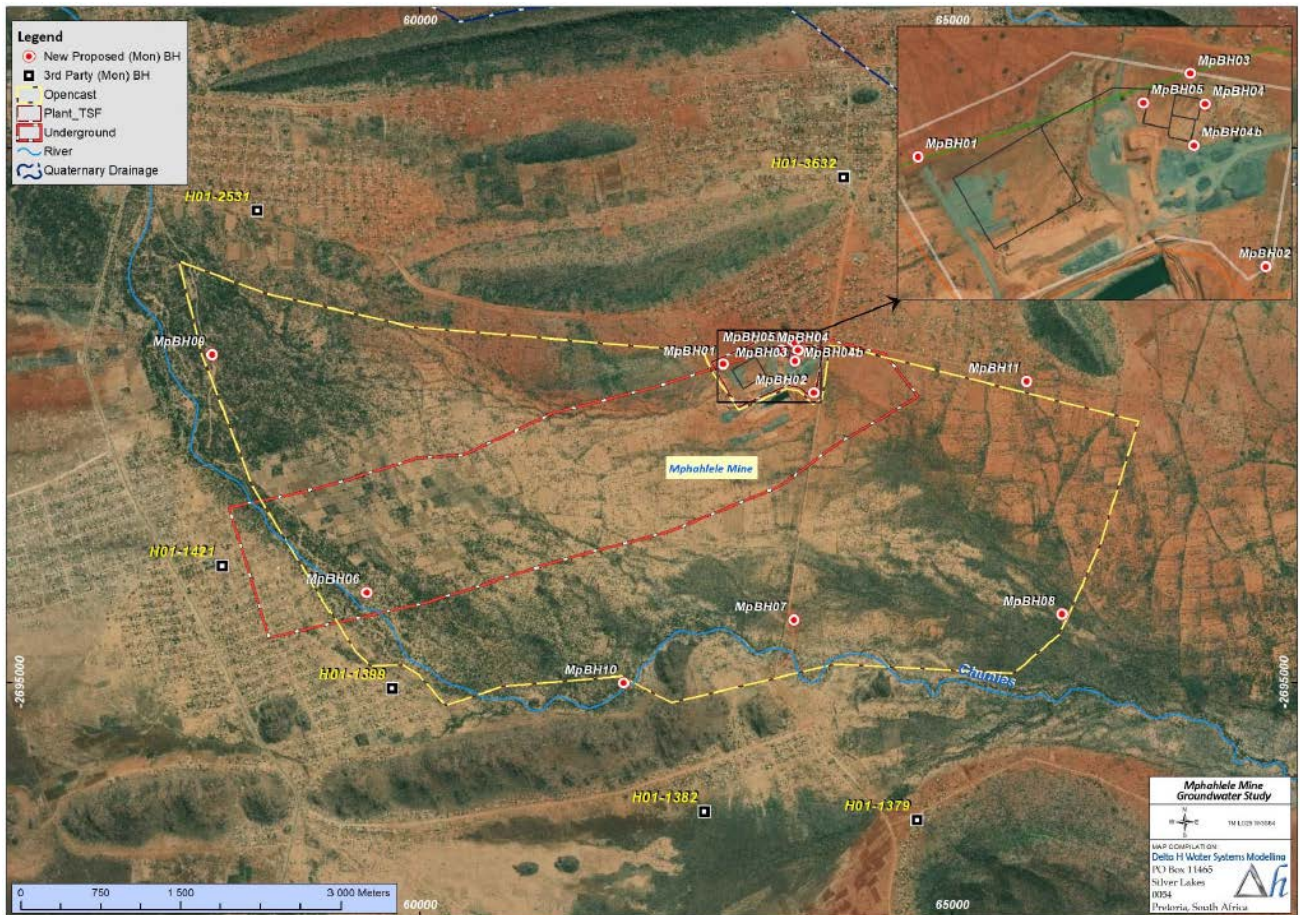
Figure 47: Proposed monitoring boreholes for the Mphahlele Mine.
