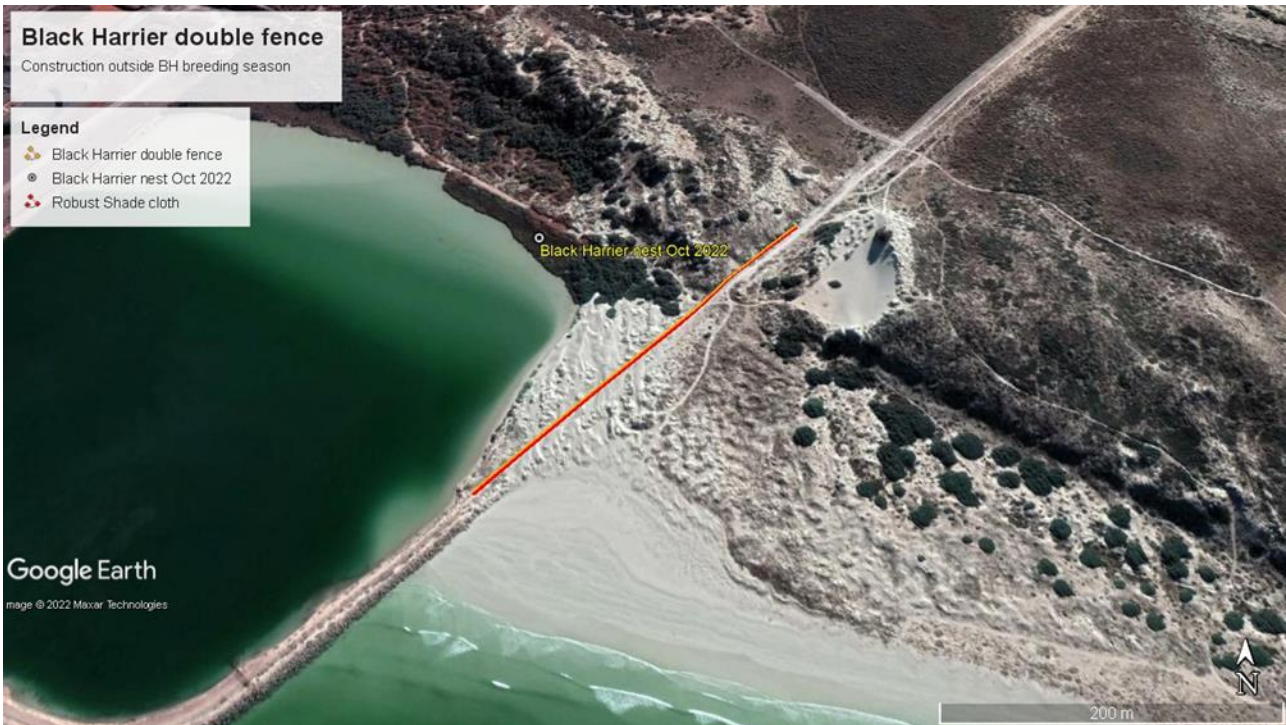
Figure 7-11: The proposed double fence around the Black Harrier nest to prevent disturbance and human intrusion from the Stringing Yard operations. The red line represents a screening fence (robust shade cloth) to reduce visual impacts over and above the chain-link fence to reduce human intrusions. The north-west side of the fence no longer joins with the Iron ore depot to allow access to wood cutters to remove alien trees smothering the two vleis here.
